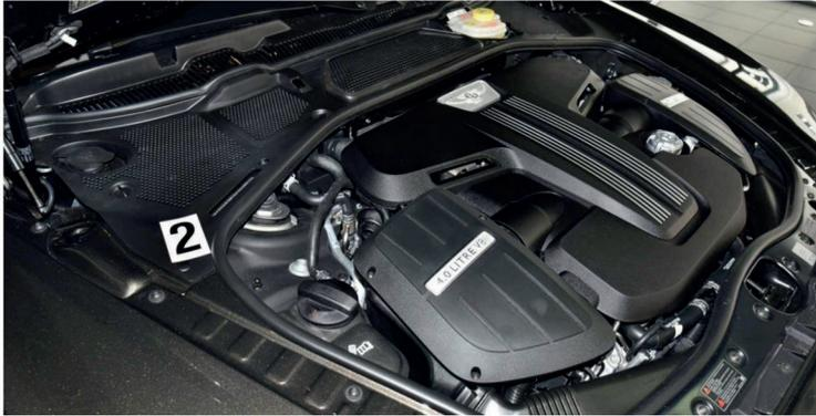
Fig. 1. A standard VIN position in the engine compartment of a Bentley Continental GT vehicle. The VIN is easily visually accessible (to the right from the number "2")
