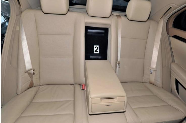
**Fig. 6. A VIN located in a non-standard way in a Mercedes – Benz "S" class vehicle in the space behind the elbow rest of the rear seats. It occurs to hardly anyone to look for the identifier there. On the other hand, this space is clean, dust-free so the identifier is not exposed to the negative effects of ambient phenomena**
