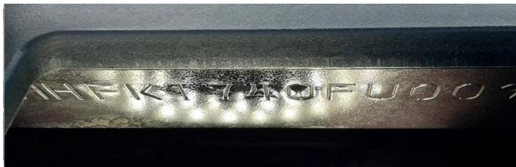
Fig. 4. Overall, the identifier is visually inaccessible even following this dismantlement. Reading the VIN is very uncomfortable, and the inclined surface plays a role as well
