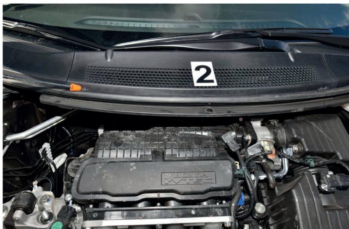
**Fig. 2. Example of a difficult-to-access VIN in a Honda Civic vehicle. For the identifier to be visually accessible, plastic parts must be expertly dismantled**
