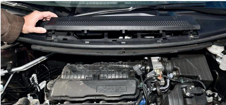
Fig. 3. Demonstration of a dismantled plastic cover in the space in front of the windscreen wipers
