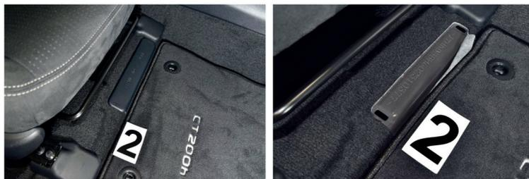
**Fig. 7. The VIN of a Lexus CT 200h vehicle standardly placed below the front passenger's seat. The VIN is protected by a plastic guard against damage and soiling**
