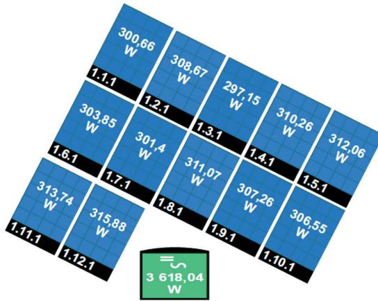
Fig. 3. Monitoring of individual photovoltaic panels
