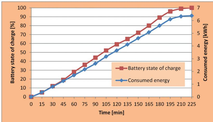
Fig. 9. The chart of the battery charging process, including energy consumption
