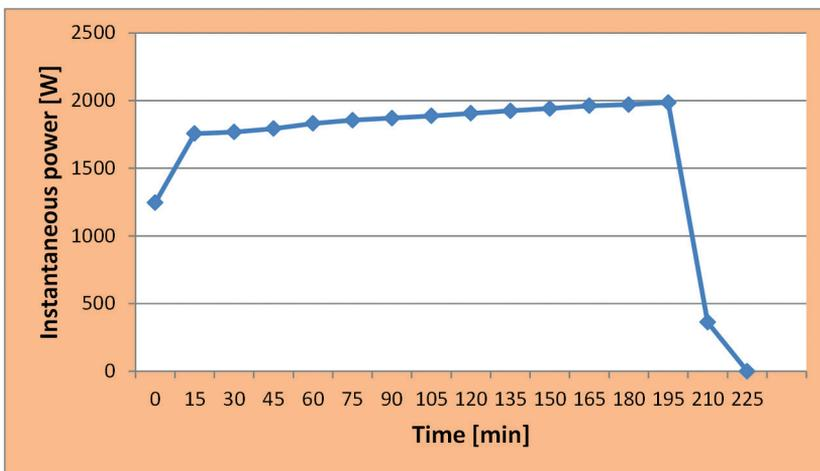
Fig. 8. The demand for electric power during charging an electric vehicle
