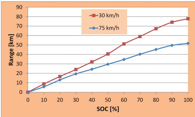
Fig. 10. The range of the small urban vehicle depending on the average driving speed
