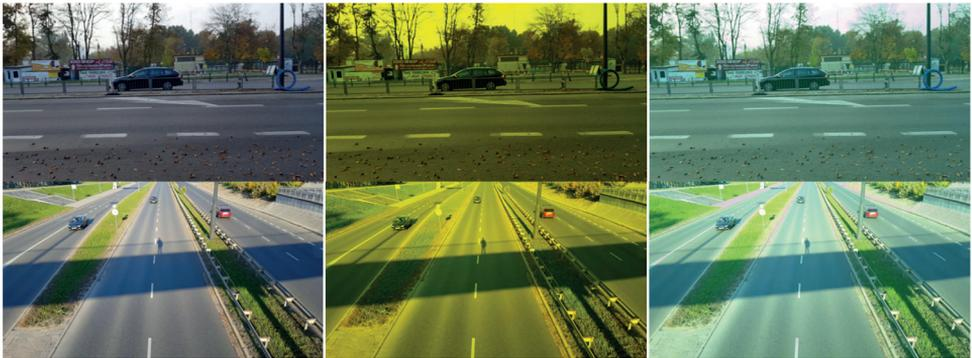
**Fig. 7. Object image - baseline, with color multiplication (blue channel removed) and with color shifted (+10,+50,+25). Author's materials**
