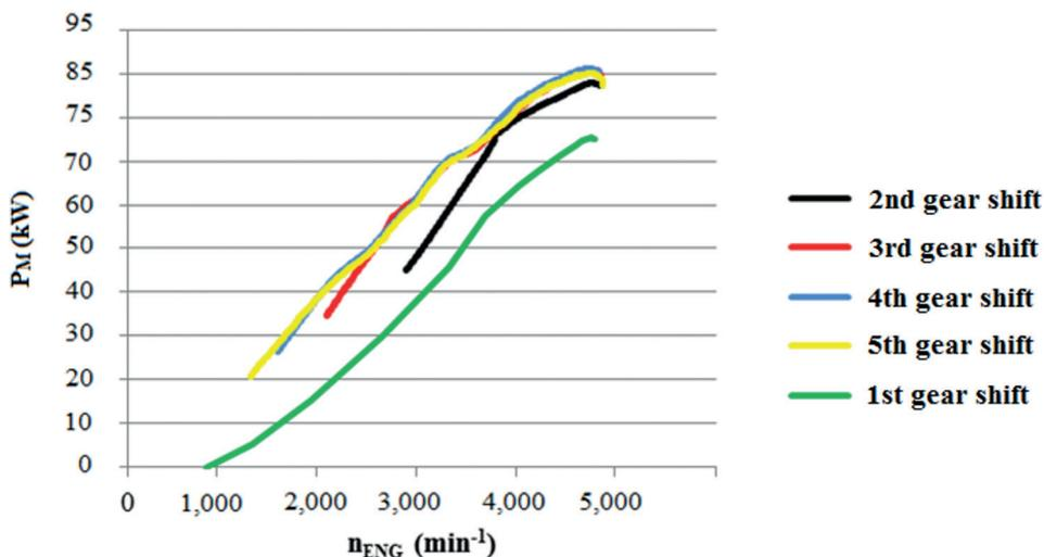
Fig. 2. Engine power curves at each gear shift. Source: authors
