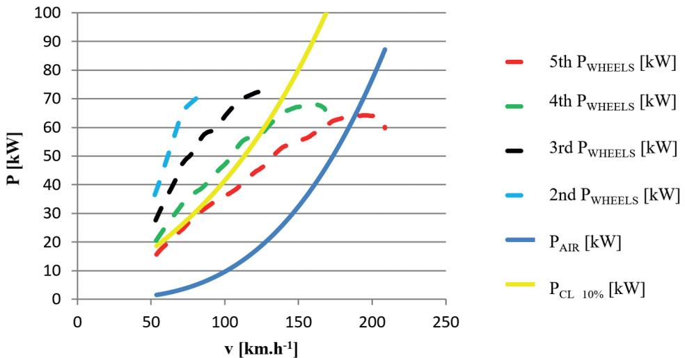
Fig. 3. Engine power curves of the tested car. Source: authors
