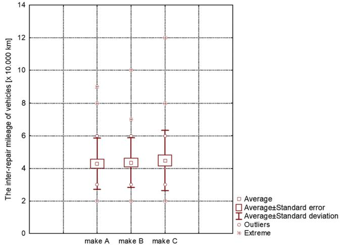
Fig. 9 The inter-repair mileage of vehicles according to the questionnaire surveys
