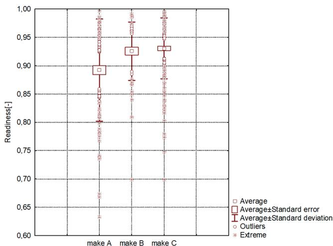
Fig. 5. Comparison of averaged readiness in the entire observed period of operation
