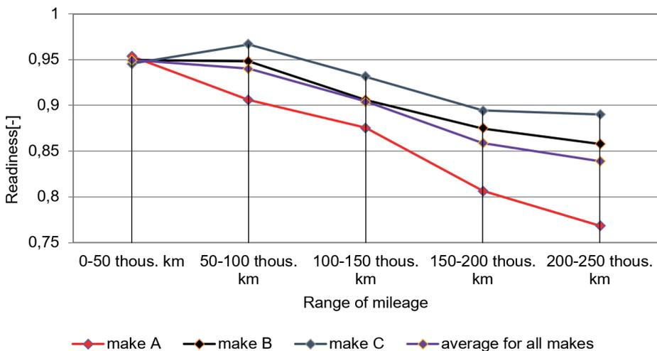
Fig. 4. Comparison of readiness changes with respect to the average for all makes
