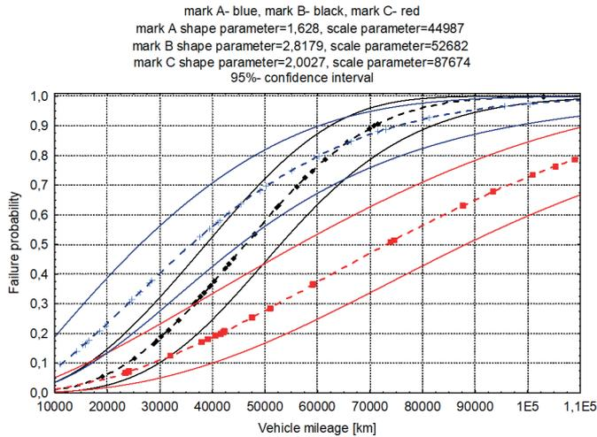
Fig. 6. Comparison of the cumulative distributions of the mileages course to the first defect
