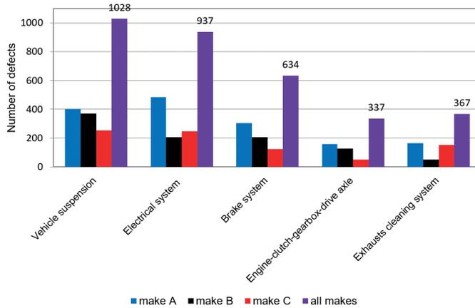
Fig. 11. List of the empirical number of repairs related to selected vehicle functional systems
