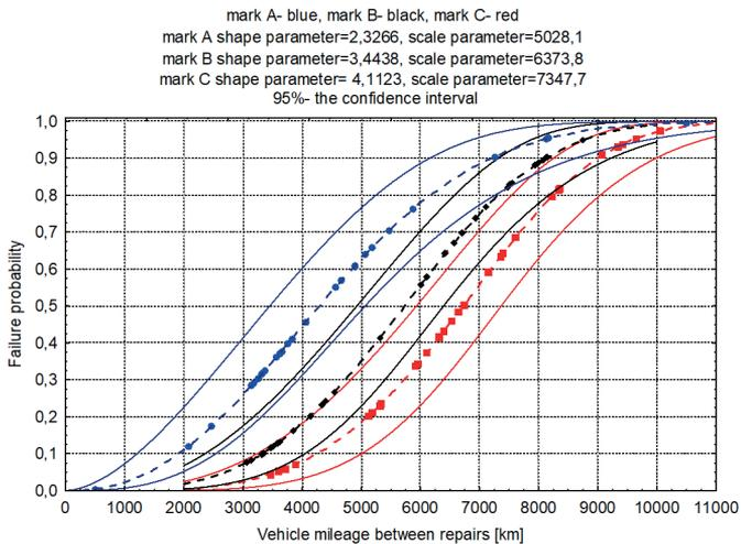
Fig. 7. Comparison of cumulative distributions of the inter-repair mileage courses
