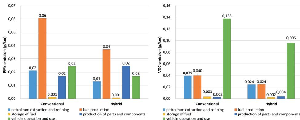
Fig. 4. Emission levels:  $\text{PM}_x$  (on the left) and VOC (on the right) for the individual phases of the life cycle of the city buses
