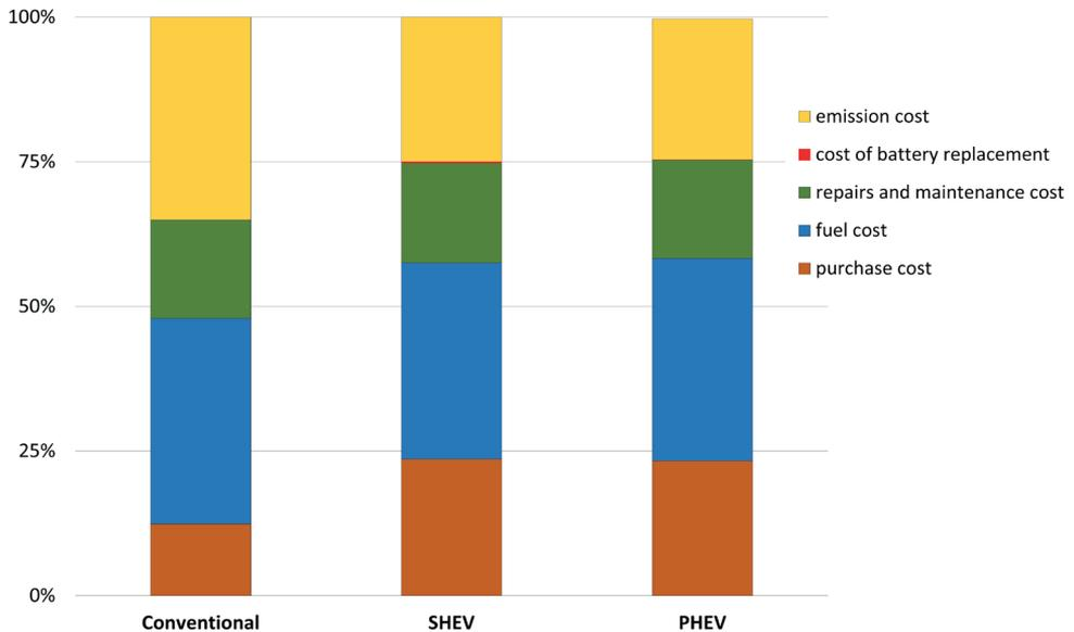
Fig. 6. Share of costs for LCC of a city bus with a conventional, hybrid series (SHEV), and hybrid parallel (PHEV) drives
