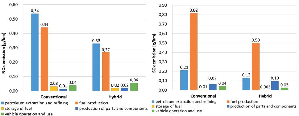
Fig. 3. Emission levels: NO<sub>x</sub> (on the left) and SO<sub>x</sub> (on the right) for the individual phases of the life cycle of the city buses
