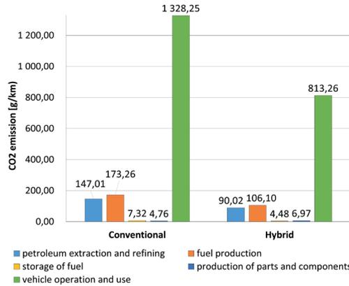
Fig. 2. CO<sub>2</sub> emissions level for individual stages of the life cycle of the conventional and hybrid bus
