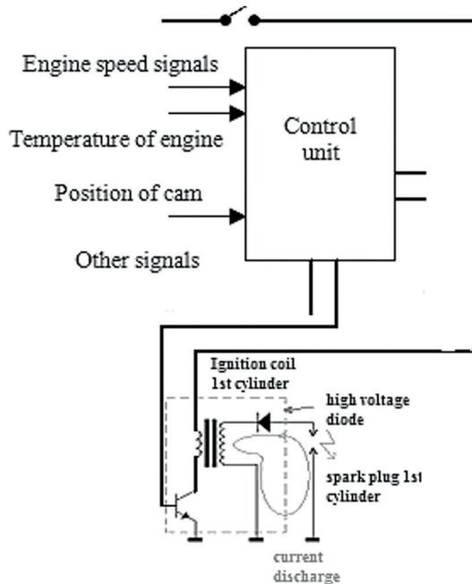
Fig. 2. Simplified EFS ignition scheme
