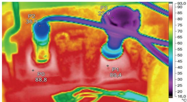
Fig. 8. Thermogram of ignition coils
