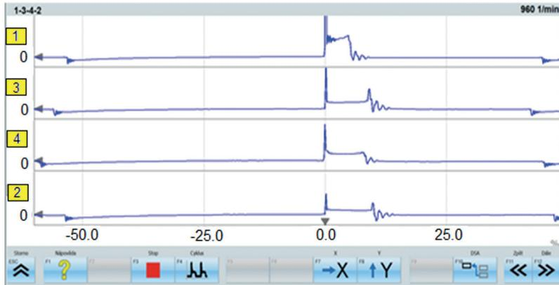
Fig. 5. Measured high-voltage spark curves - the primary side of ignition
