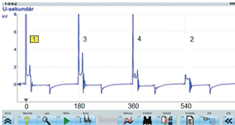
Fig. 7. Measured high-voltage ignition curves due to defective spark plug
