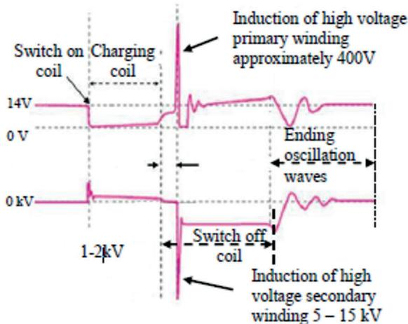
Fig. 1. Voltage waveforms of the primary side of the transformer winding
