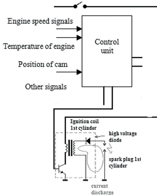
Fig. 2. Simplified EFS ignition scheme
