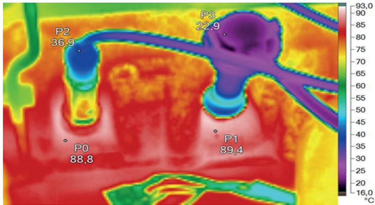
Fig. 8. Thermogram of ignition coils
