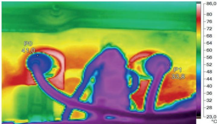
Fig. 3. Thermogram ignition coil 1st and 2nd cylinders
