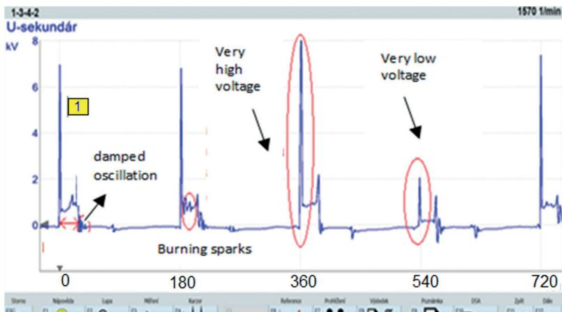
Fig. 6. Measured high-voltage ignition curves with faulty spark plugs
