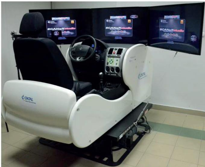
Fig. 1. Driver compartment on the motion platform and the monitors
