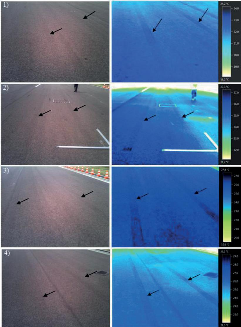
Fig. 2. Thermal image of skid mark [6]
