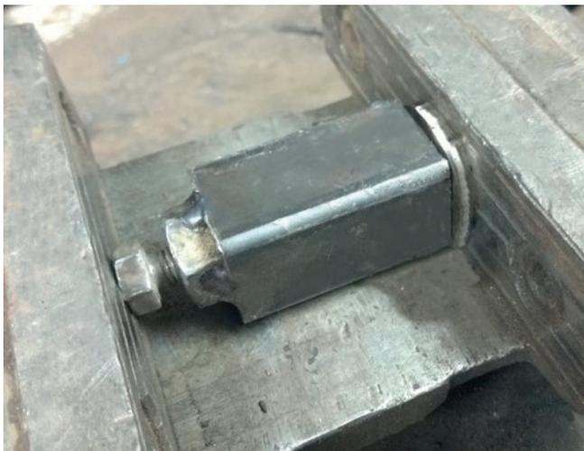
Fig. 4. Die for cold working process
