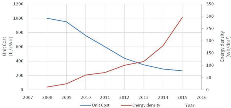
Fig. 2. Unit cost (€/kWh) and energy density (Wh/dm<sup>3</sup>) of lithium-ion batteries
