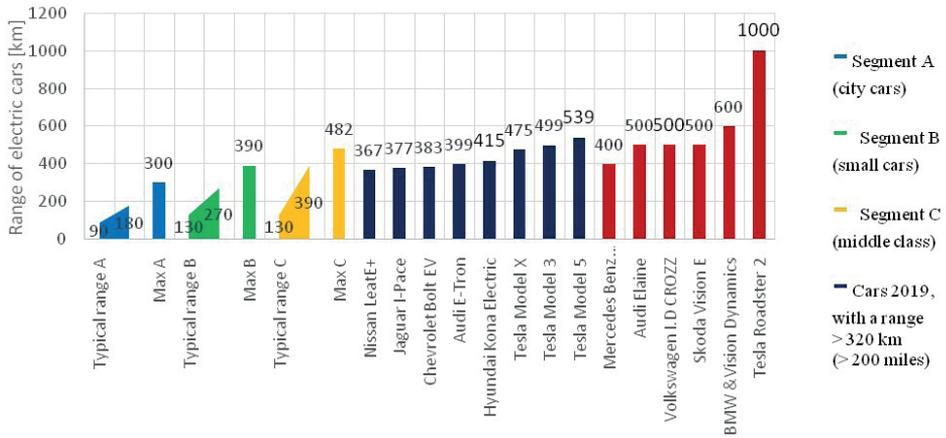
Fig. 3. The range of selected electric cars.
