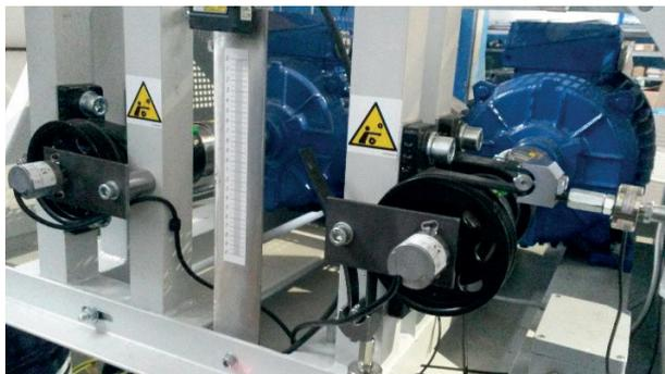
Fig. 1. Research stand for measuring friction parameters of a belt transmission
