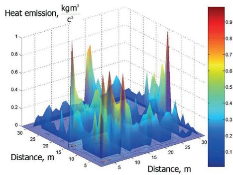
b) The equivalent level of heat emission (final version) at the flow density 0.9
