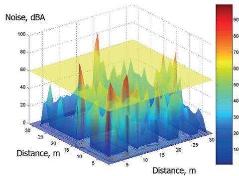
b) The equivalent level of noise (final version) at the flow density 0.8
