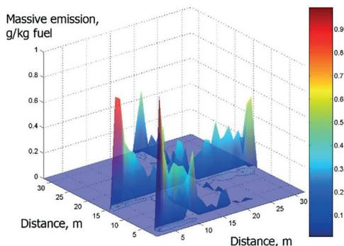
a) The equivalent level of gas pollution (parent version) at the flow density 0.9
