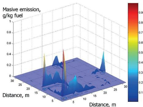
b) The equivalent level of gas pollution (final version) at the flow density 0.9
