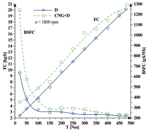
Fig. 3. Load characteristics of Perkins 1104D-E44TA engine determined for crankshaft speed  $n=1800$  rpm, powered by compressed natural gas and diesel (CNG+D) in dual-fuel operation and by diesel fuel (D) only
