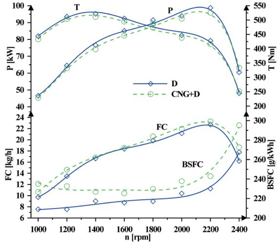
Fig 2. External speed characteristics of Perkins 1104D-E44TA engine running on compressed natural gas and diesel fuel (CNG+D) in dual-fuel operation and on diesel fuel (D) only
