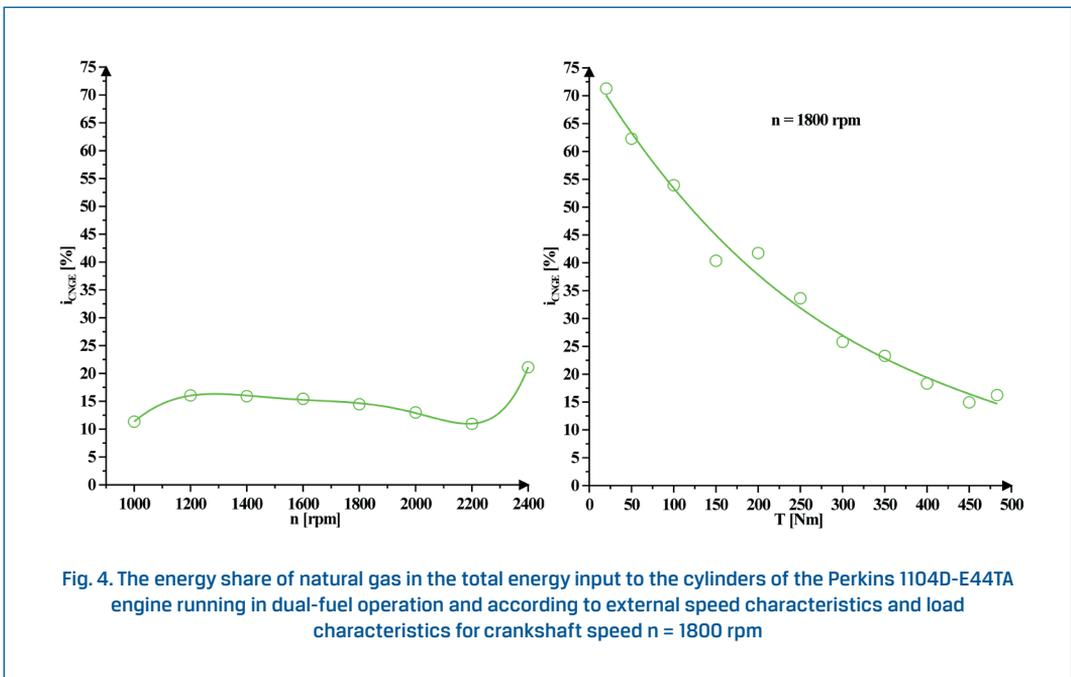
Fig. 4. The energy share of natural gas in the total energy input to the cylinders of the Perkins 1104D-E44TA engine running in dual-fuel operation and according to external speed characteristics and load characteristics for crankshaft speed  $n = 1800$  rpm
