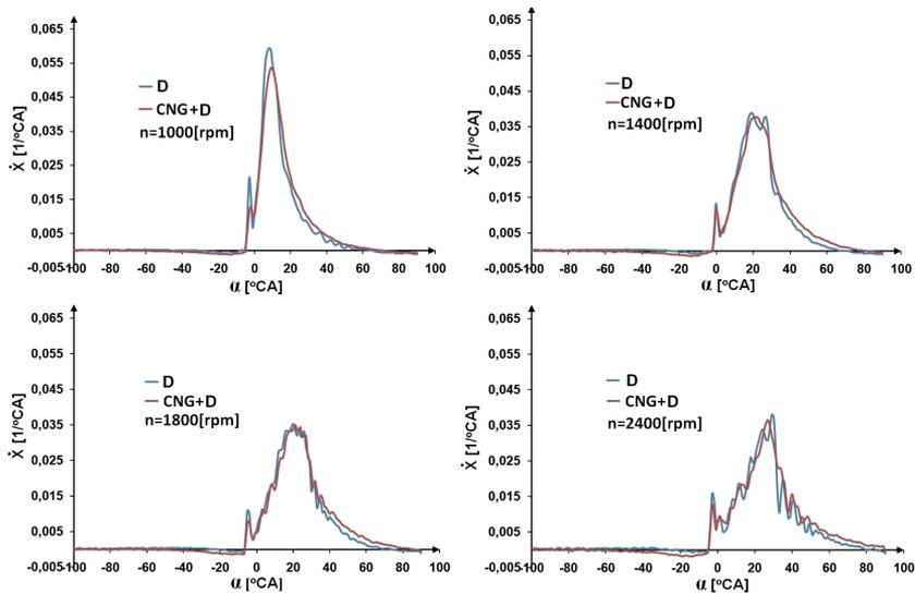
Fig. 8. The rate of relative amount of heat released during the combustion process in the Perkins 1104D-E44TA engine cylinder powered by compressed natural gas and diesel (CNG+D) and by diesel fuel (D) only, operating according to external speed characteristics, at selected crankshaft speeds  $n$
