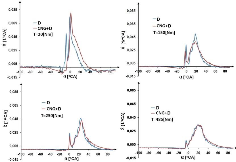
Fig. 9. The rate of relative amount of heat released during the combustion process in the Perkins 1104D-E44TA engine cylinder powered by compressed natural gas and diesel (CNG+D) and by diesel fuel (D) only, operating according to the load characteristics for crankshaft speed  $n = 1800$  rpm, at selected loads determined by the value of torque  $T$
