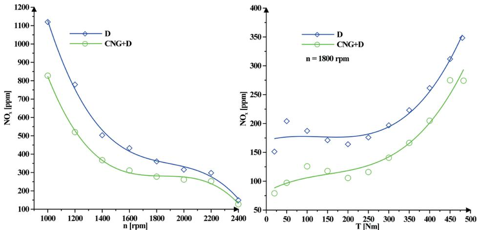
Fig. 5. Comparison of the concentrations of nitrogen oxides in the exhaust gas of a Perkins 1104D-E44TA engine running on compressed natural gas and diesel (CNG+D) in dual-fuel operation and when powered by diesel (D) only, operating according to the external speed characteristics and according to the load characteristics for crankshaft speed  $n = 1800$  rpm
