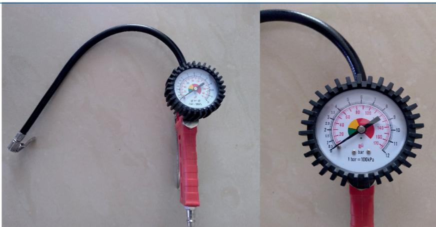
Fig. 4. Clock manometer used to measure the pressure value
