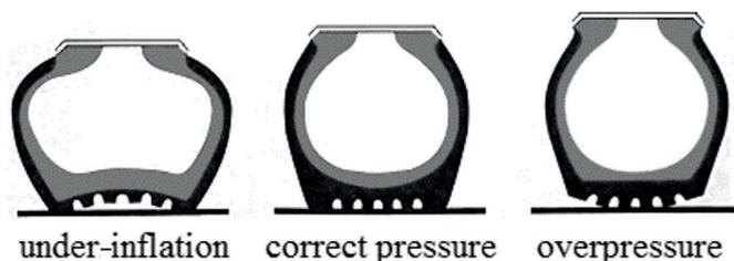
Fig. 1. Pressure values in the tire dependent on the contact surface
