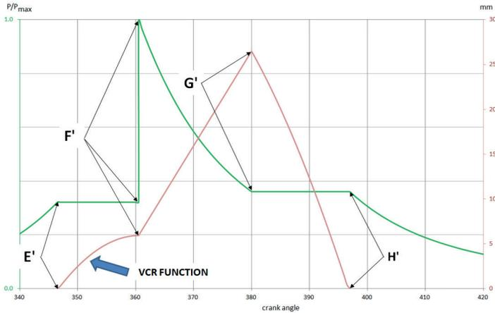
Fig. 11. Four characteristic points of work for theoretical cycle of ACC engine
