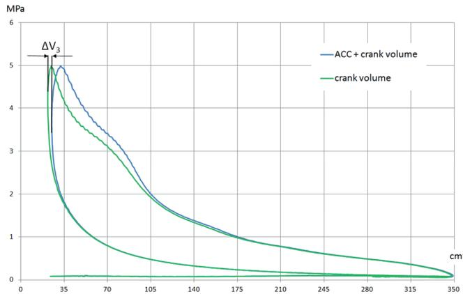
Fig. 8. Pressure volume diagram of the crank-piston system volume and cumulative volume (optimal reaction of ACC system)
