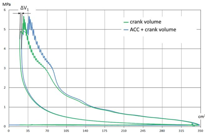
**Fig 6. Pressure volume diagram of the crank-piston system volume and cumulative volume (delayed reaction of ACC system, 70% loading)**
