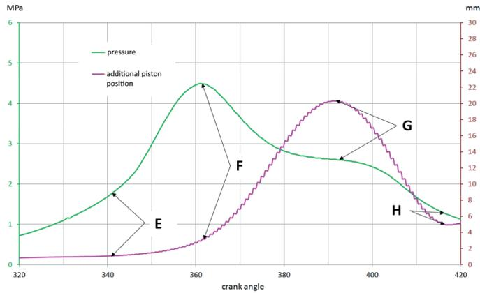
Fig 9. Four (E, F, G, H) characteristic points for real ACC engine subjected to partial load
