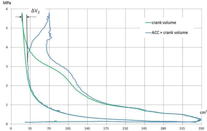
Fig. 7. Pressure volume diagram of the crank-piston system volume and cumulative volume (premature reaction of ACC system, 80% loading)
