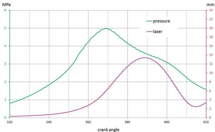
Fig. 4. Optimal pressure course and displacement of additional piston in ACC engine with VCR function
