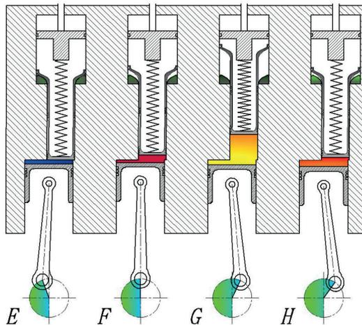
Fig. 10. Four (E, F, G, H) characteristic points of ACC engine
