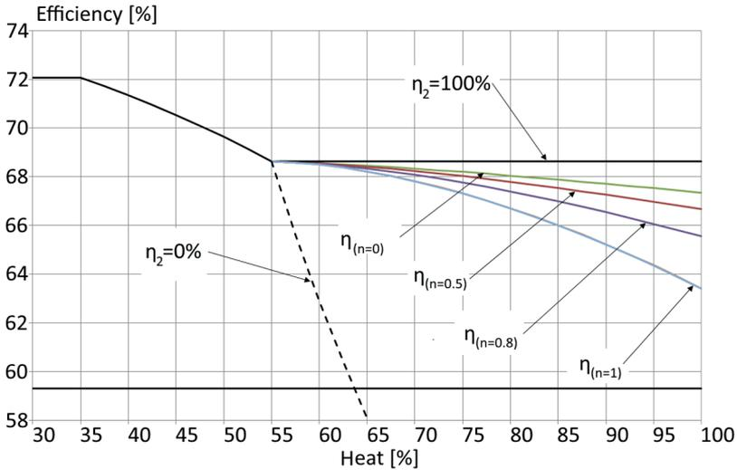
Fig. 13. Efficiency of the new Otto cycle as a function of load
