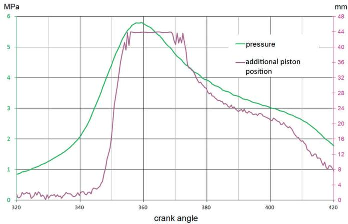
Fig. 3. Indicated pressure and displacement of the additional piston for an premature ACC system reaction
