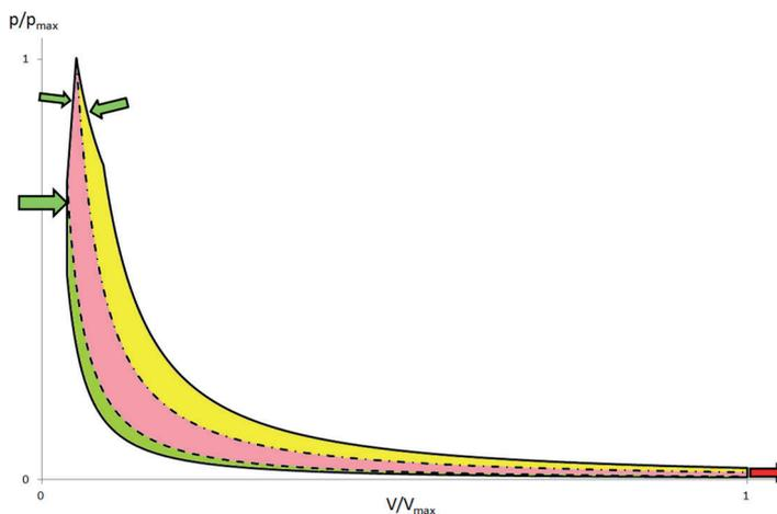
Fig. 17. Theoretical cycle of ACC engine with premature response
