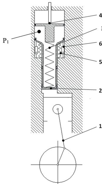
Fig. 1. Schematic diagram of ACC engine operation
