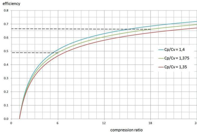
Fig. 5. Otto cycle efficiency as a function of compression ratio
