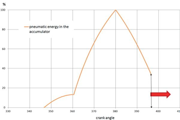
Fig. 16. The course of energy accumulation and recuperation in theoretical (frictionless) ACC system
