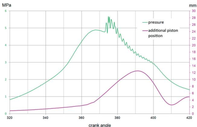
Fig. 2. Indicated pressure and additional piston movement for delayed reaction of ACC system
