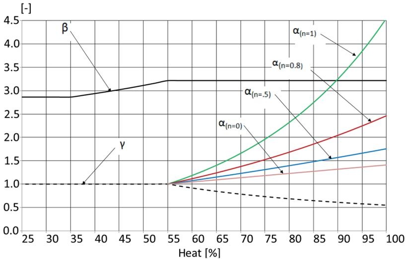
Fig. 14. Change of values for  $\alpha$ ,  $\beta$  and  $\gamma$  factors as a function of load
