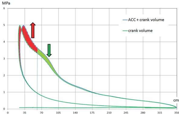
Fig. 15. Real energy balance for ACC system with VCR function for closed cycle
