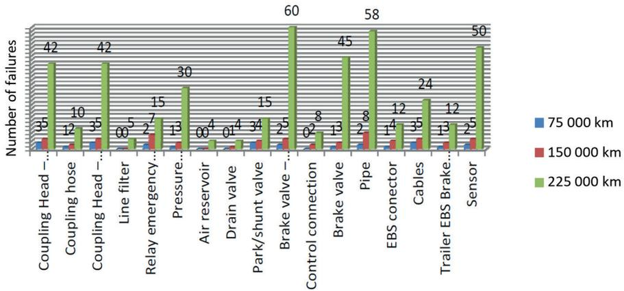
Fig. 1. The number of failures of the components of the air brake system
