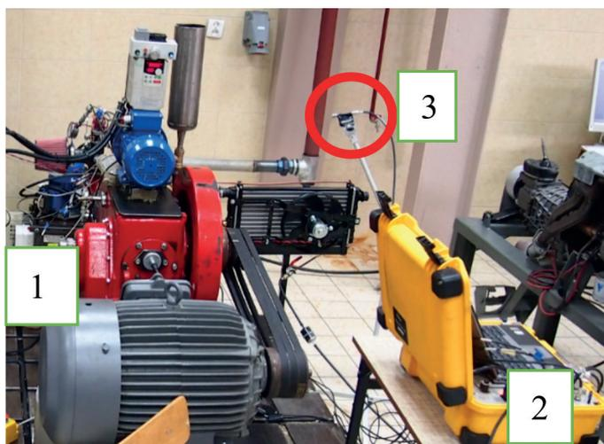
**Fig. 1. Engine sound pressure measurement stand: 1 - Andoria Diesel engine S320 with CELMA Type 2Sf200 LG/4A electric starter-generator; 2 - Bruel & Kjaer sound record equipment; 3 - microphone**
