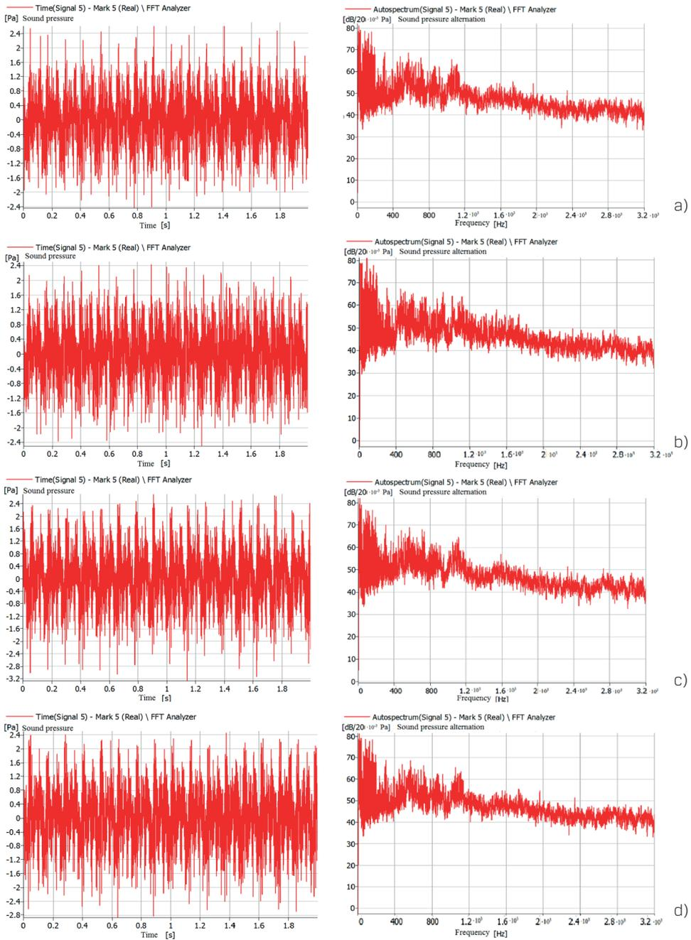
**Fig. 2.** The graphs of sound pressure and its spectral density were varied with power under different operating conditions: a – 2.63 kW; b – 4.8 kW; c – 6.56 kW; d – 9.48 kW
