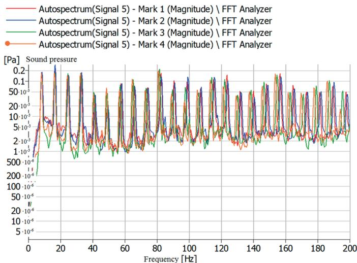
Fig. 3. Graph of sound pressure spectral density under different operating conditions (variable power 2.63 kW, 4.8 kW, 6.56 kW and 9.48 kW) with frequency range up to 200 Hz
