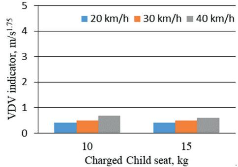
Fig. 13. VDV values of the accelerations registered on the seat of the "B" car child seat
