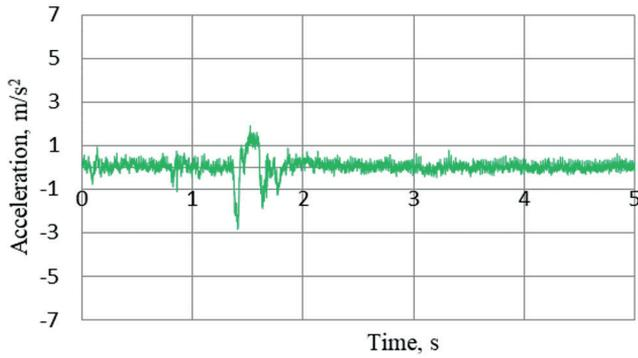
**Fig. 8.** Effective values of accelerations registered on the seat of the "A" car child seat, during driving car through the deceleration speed bump at a speed of 20 km/h, child seat charged of mass 10 kg
