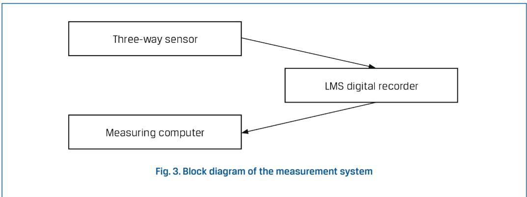
In the conducted tests, the measured values were accelerations: car rear seats, seats and backrests of the tested child seats and the ISOfix base, which were measured using four three-directional acceleration sensors (Table 1).
