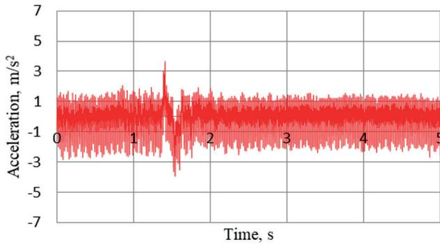
Fig. 7. Effective values of accelerations registered on the basis of ISOfix, during driving car through the deceleration speed bump at a speed of 20 km/h and charged of mass 10 kg on seat of "A" car child seat
