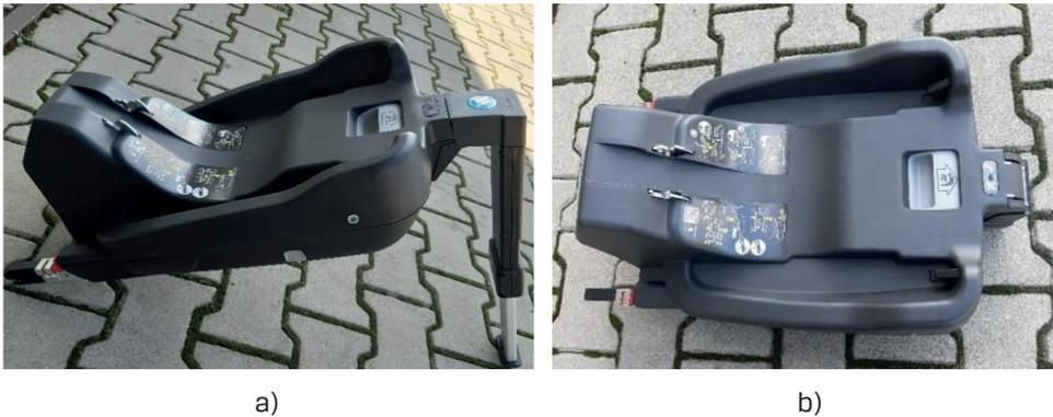
**Fig. 1. View of base ISOfix used: a) base with unfolded stabilizing support, b) base with a complex stabilizing support**
