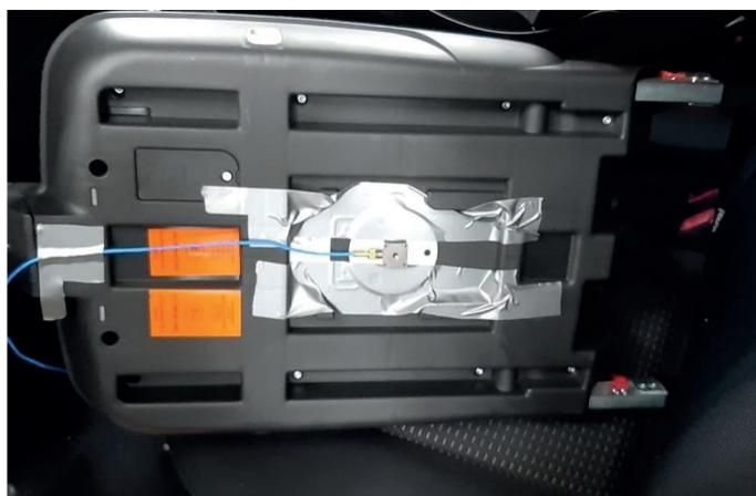
Fig. 5. Location and method of mounting the three-directional acceleration sensor based on ISOfix
