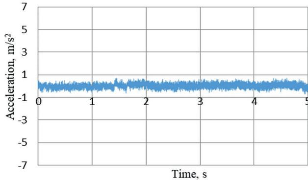
Fig. 6. Effective values of accelerations registered on the rear seat of the car, during driving car through the deceleration speed bump at a speed of 20 km/h, seat charged of mass 10 kg
