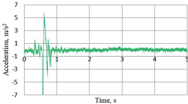
Fig. 11. Effective values of accelerations registered on the seat of the "A" car child seat, during driving car through the deceleration speed bump at a speed of 40 km/h, child seat charged of mass 10 kg
