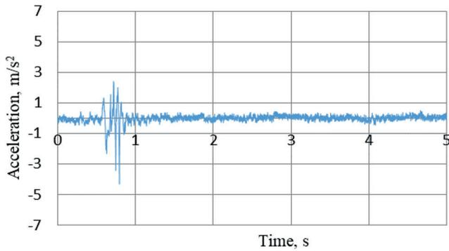
**Fig. 9.** Effective values of accelerations registered on the rear seat of the car, during driving car through the deceleration speed bump at a speed of 40 km/h, seat charged of mass 10 kg
