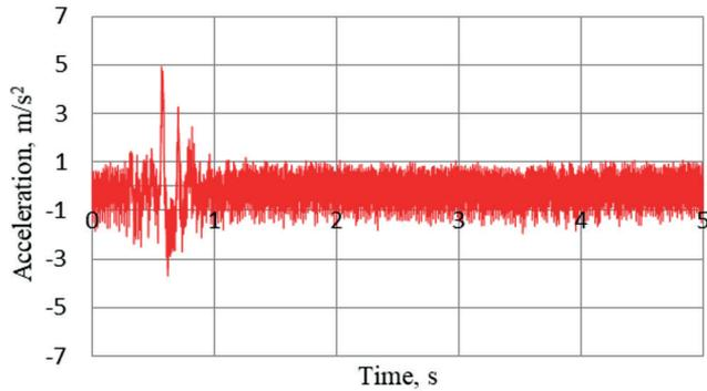
Fig. 10. Effective values of accelerations registered on the basis of ISOfix, during driving car through the deceleration speed bump at a speed of 40 km/h and charged of mass 10 kg on seat of "A" car child seat
