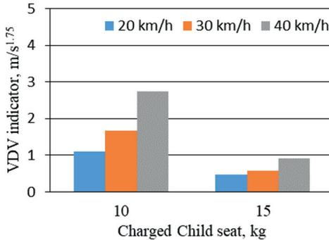
Fig. 12. VDV values of the accelerations registered on the seat of the "A" car child seat
