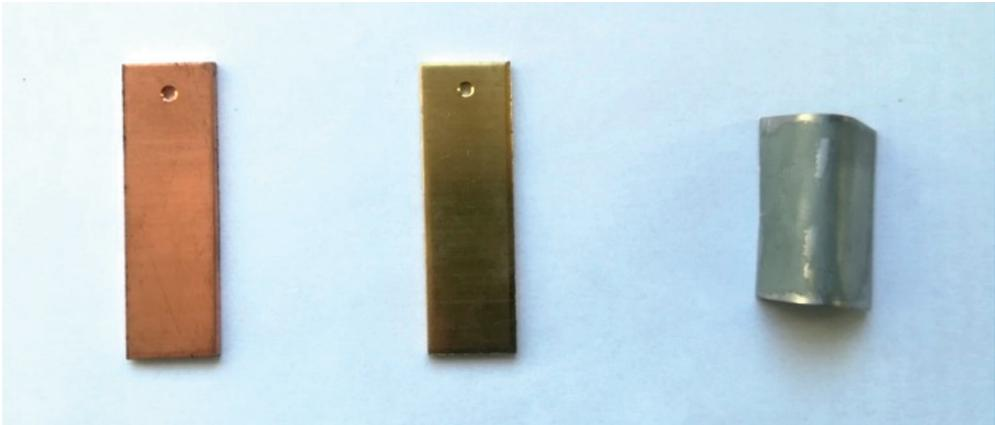
Fig. 1. Metal plates used in the tests: 1) copper; 2) brass; 3) zinc
