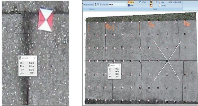
Fig. 8. Measurement of the deviation between reference raster and raster after rectification [10]
