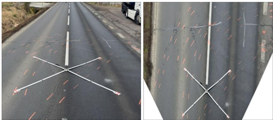
Fig. 4. Photography before rectification (left) and after rectification (right)
