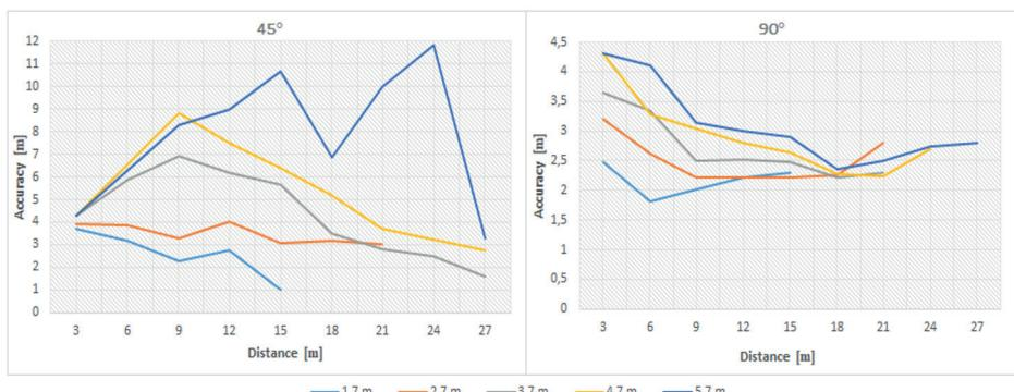
Fig. 10. Comparison of accuracy for rectification method for deviation not bigger than 20 cm for different position of rectification cross (45° and 90°) [9]
