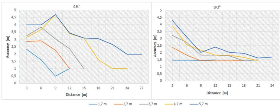
Fig. 9. Comparison of accuracy for rectification method for deviation not bigger than 10 cm for different position of rectification cross (45° and 90°) [9]
