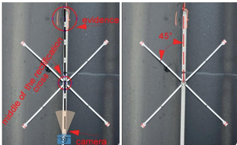
Fig. 2. Position of the rectification cross towards to the evidence
