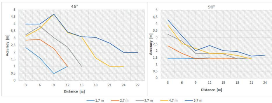
Fig. 9. Comparison of accuracy for rectification method for deviation not bigger than 10 cm for different position of rectification cross ( $45^\circ$  and  $90^\circ$ ) [9]
