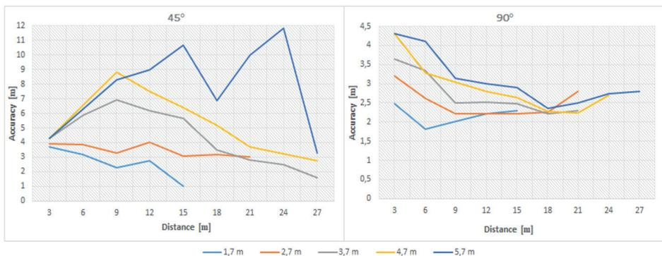
Fig. 10. Comparison of accuracy for rectification method for deviation not bigger than 20 cm for different position of rectification cross ( $45^\circ$  and  $90^\circ$ ) [9]
