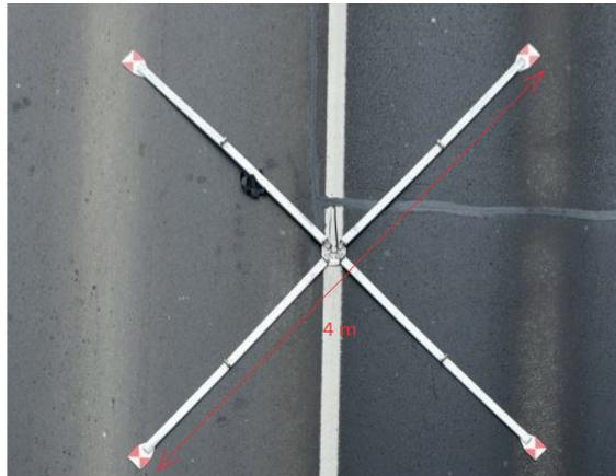
Fig. 1. Rectification cross with rectification targets
