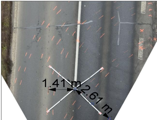
Fig. 5. Measurement of the distance from photography after rectification in PC Crash
