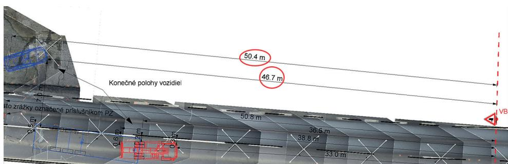
**Fig. 7.** In the red circle are distance measured in PC-Crash from rectified photography
