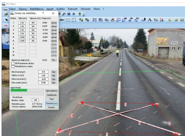
Fig. 3. Rectification window in PC Rect
