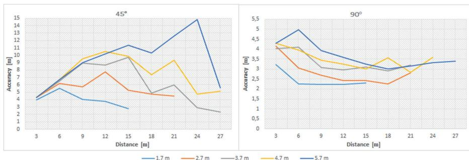
Fig. 11. Comparison of accuracy for rectification method for deviation not bigger than 30 cm for different position of rectification cross (45° and 90°) [9]
