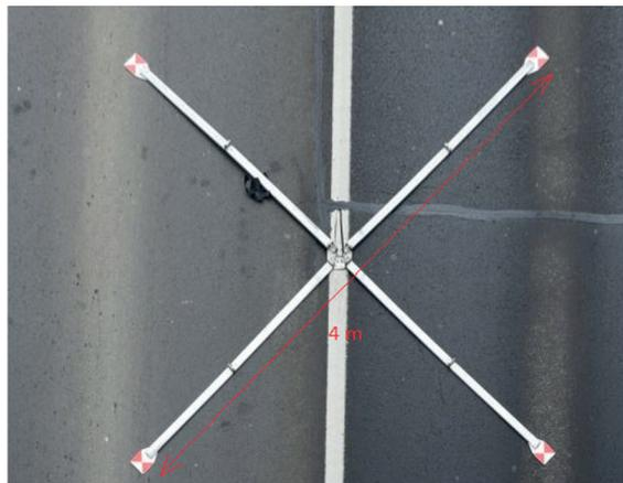
Fig. 1. Rectification cross with rectification targets
