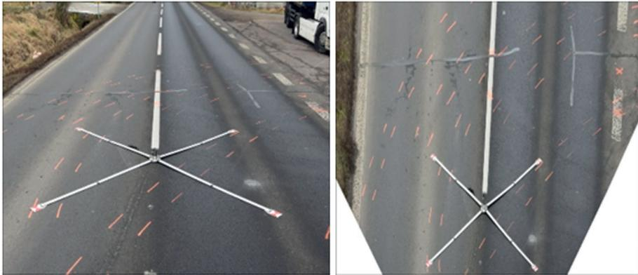
Fig. 4. Photography before rectification (left) and after rectification (right)
