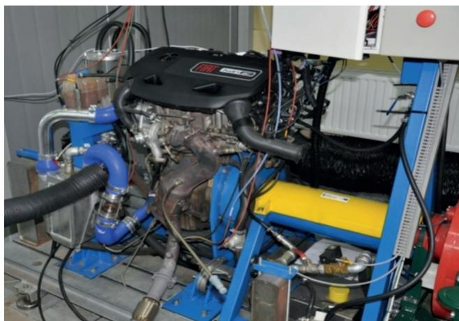
Fig. 1. View of the Fiat 0.9 TwinAir engine test bench
