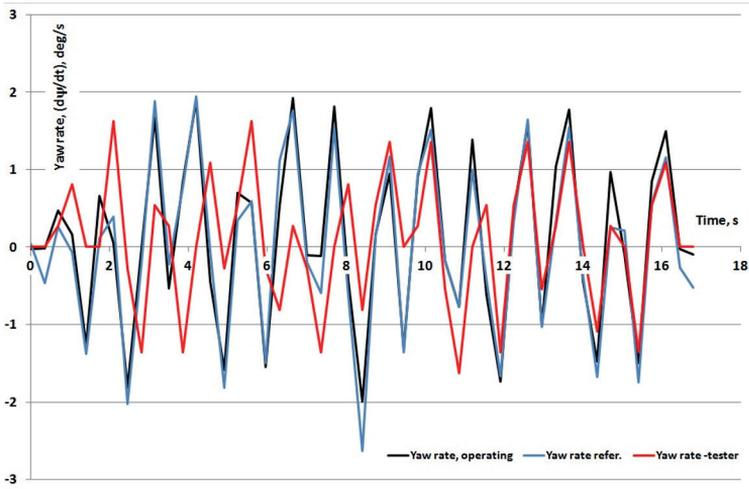
Fig. 10. Runs of yaw rate  $d\psi/dt$ , recorded in the test No. 433; the steering wheel free
