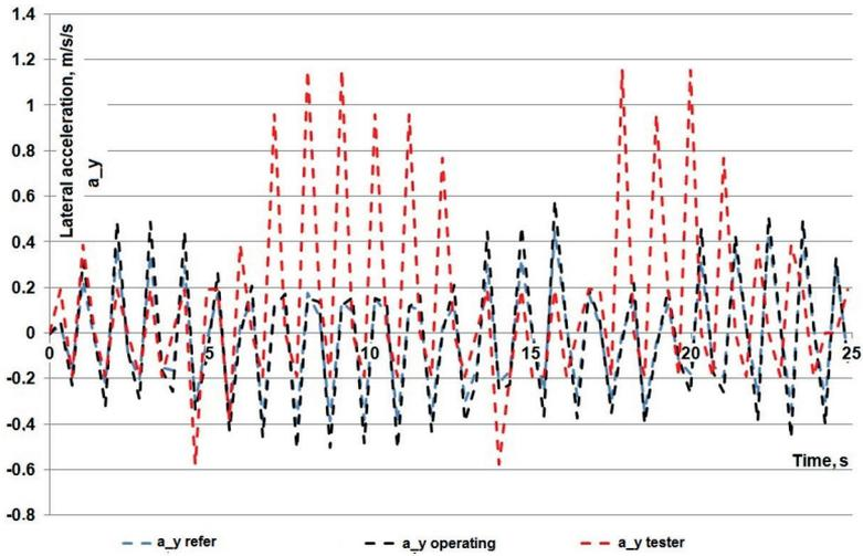
Fig. 13. Runs of lateral acceleration  $a_y$ , recorded in the test No. 435; the steering wheel fixed
