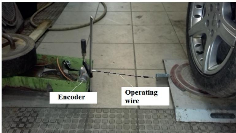
Fig. 7. View of a component part of the test stand. Rear wheels of vehicle are placed on rotary and sliding plates. The picture shows a draw-wire encoder connected with the plate under the left wheel of vehicle
