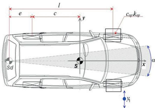
Fig. 1. Simplified model of a vehicle positioned at a wheel play detector stand.  $S$  - Vehicle mass center;  $e$  - Distance of hypothetical angular vibration center  $S_d$ ,  $c_{op}$  - coefficient of tire lateral stiffness,  $k_{op}$  - coefficient of tire lateral damping,  $\alpha_1$  - amplitude of car angular displacement relative to  $S_d$
