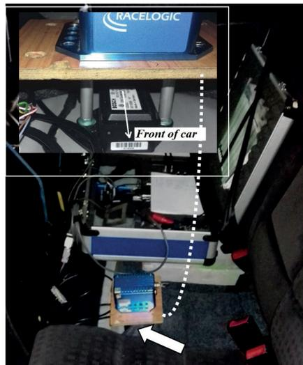
Fig. 2. Measuring apparatus located inside a tested car. The reference sensor – six-parameters measuring IMU block of Vbox 3i unit, RACELOGIC. The arrow points the operating sensor location underneath a rear seat. Upper part of this figure presents an apparatus set: IMU and operating sensor in real position during measurement. Pointed line is auxiliary only
