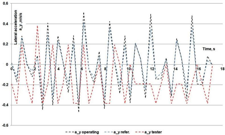
Fig. 11. Runs of lateral acceleration  $a_y$ , recorded in the test No. 434; the steering wheel fixed
