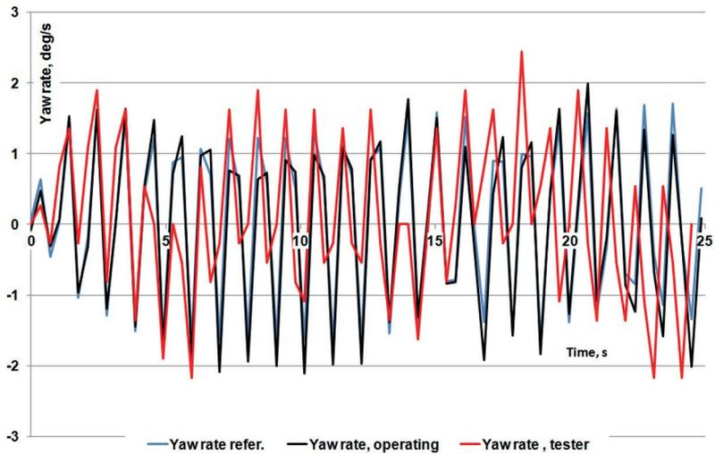
Fig. 14. Runs of yaw rate  $d\psi/dt$ , recorded in the test No. 435; the steering wheel fixed
