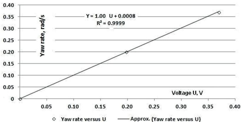
**Fig. 3. Determination of scale factor for yaw velocity measured on operating ESP sensor.
