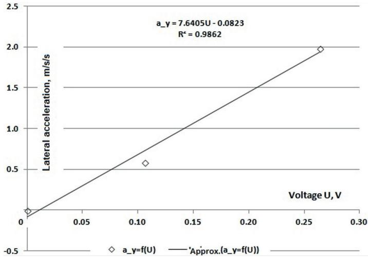
Fig. 4. Determination of scale factor for lateral acceleration measured on operating ESP sensor. The determined value is 7.64 m/s/s/Volt
