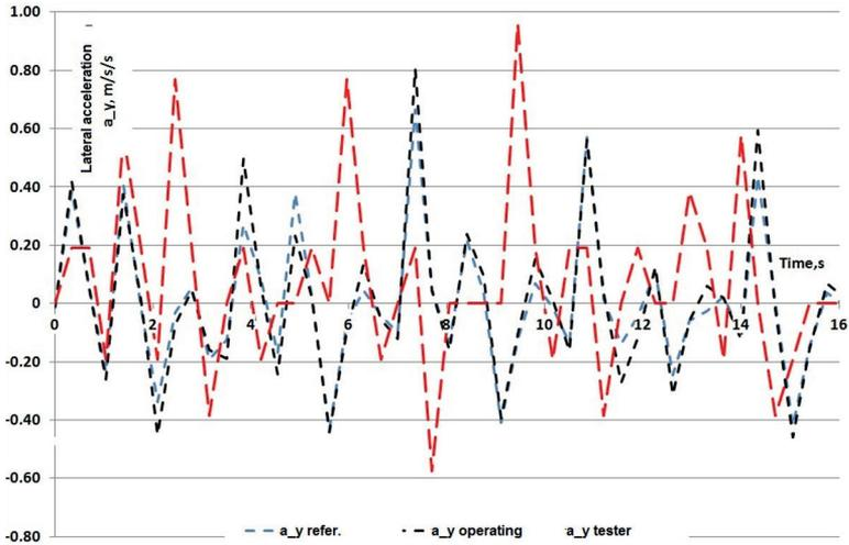
Fig. 9. Runs of lateral acceleration  $a_y$ , recorded in the test No. 433; the steering wheel freely rotating
