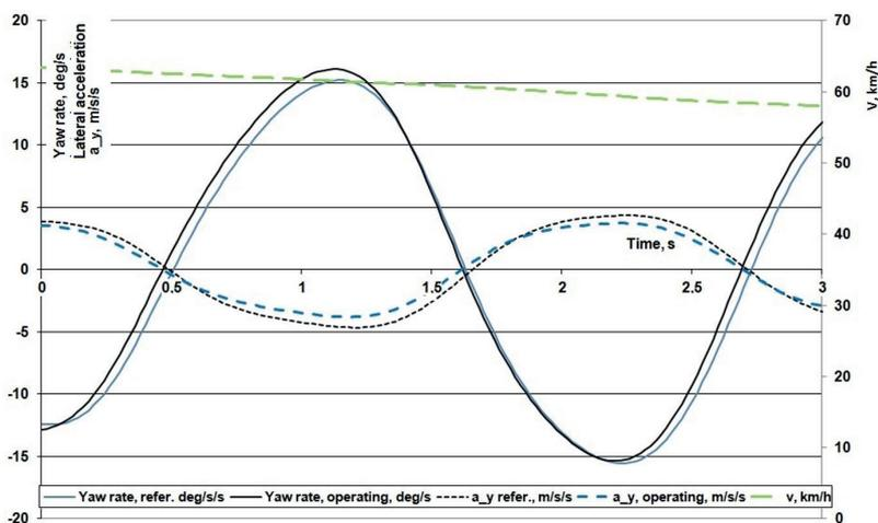
Fig. 6. Fragment of the exemplary continuous sinusoidal test from Figure 5 shown in the time interval 1 s to 3 s
