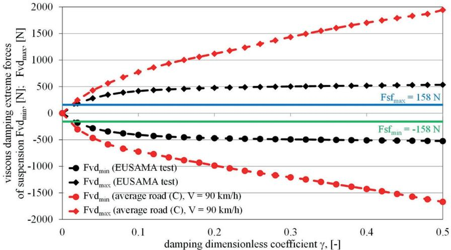
Fig. 7. Comparison of the example extremums of the viscous damping forces ( $F_{vd_{min}}$  and  $F_{vd_{max}}$ ) and sliding friction forces ( $F_{sf_{min}}$  and  $F_{sf_{max}}$ ) in the vehicle suspension system at various values of the dimensionless coefficient of damping in the suspension system (results of a simulation of the EUSAMA test and a test of vertical vibration of the vehicle on an average road (C pavement category) for a front "quarter" of the Isuzu D-max motor vehicle)
