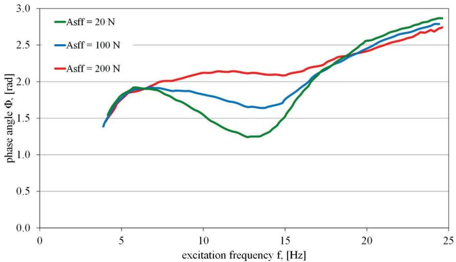
Fig. 2. Example results of diagnostic testing of the rear suspension system of an Opel Agila 1.2 Twinport with using the phase angle method, for a shock absorber in a very good condition, at a nominal and raised sliding friction in the suspension system (Asff = 20 N, Asff = 100 N and Asff = 200 N, respectively)
