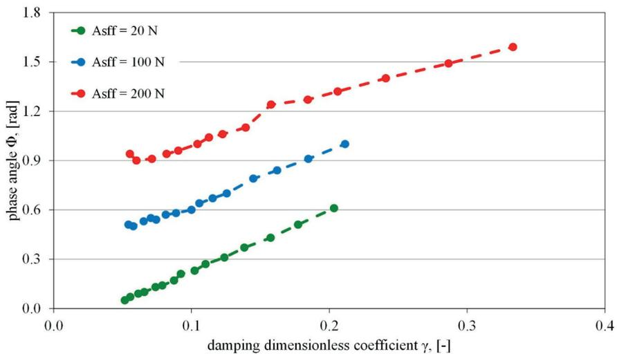
Fig. 3. Example results of diagnostic testing of the rear suspension system of an Opel Agila 1.2 Twinport with using the phase angle method, for various levels of viscous damping in the shock absorber, at a nominal and raised sliding friction in the suspension system (Asff = 20 N, Asff = 100 N and Asff = 200 N, respectively)
