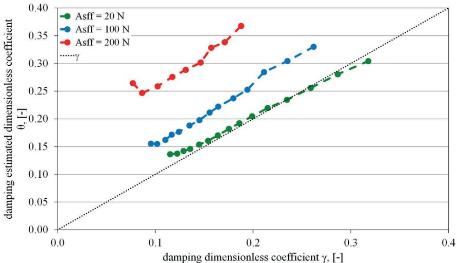
Fig. 4. Example results of diagnostic testing of the rear suspension system of an Opel Agila 1.2 Twinport with using the half power bandwidth method (HPBM), for various levels of viscous damping in the shock absorber, at a nominal and raised sliding friction in the suspension system ( $Asff = 20$  N,  $Asff = 100$  N and  $Asff = 200$  N, respectively)
