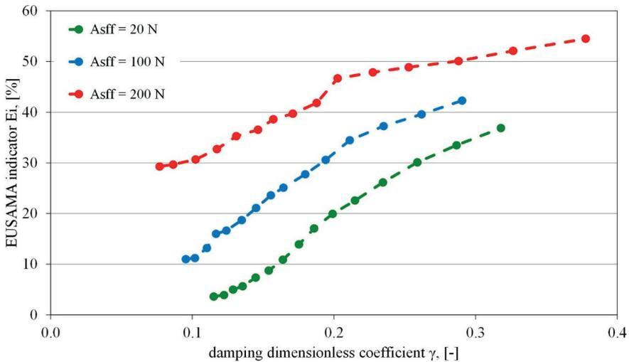
Fig. 1. Example results of diagnostic testing of the rear suspension system of an Opel Agila 1.2 Twinport with using the EUSAMA method, for various levels of viscous damping in the shock absorber, at a nominal and raised sliding friction in the suspension system ( $As_{ff} = 20$  N,  $As_{ff} = 100$  N and  $As_{ff} = 200$  N, respectively)
