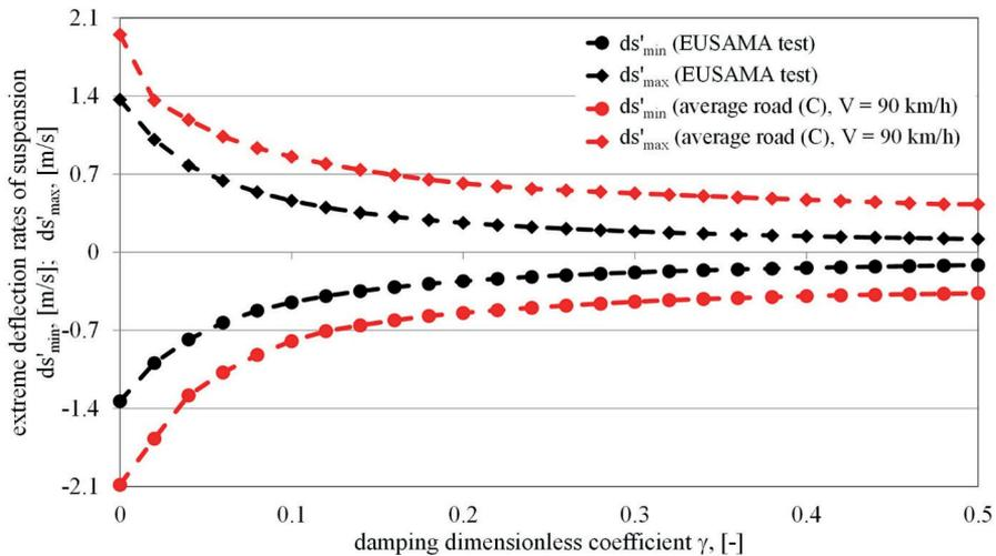
Fig. 6. Comparison of the example extremums of the deflection rates ( $ds'_{\min}$  and  $ds'_{\max}$ ) in the vehicle suspension system at various values of the dimensionless coefficient of damping in the suspension system (results of a simulation of the EUSAMA test and a test of vertical vibration of the vehicle on an average road (C pavement category) for a front "quarter" of the Isuzu D-max motor vehicle)
