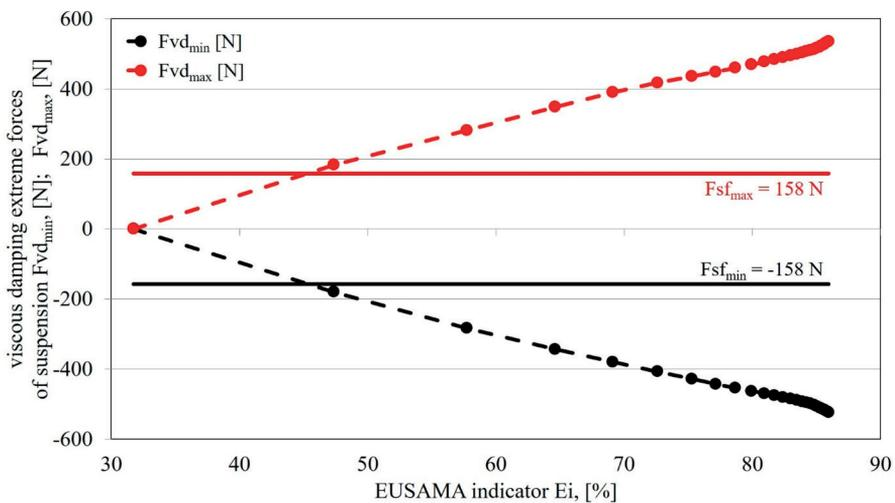
Fig. 5. Example extremums of the viscous damping forces ( $F_{vd_{min}}$  and  $F_{vd_{max}}$ ) and sliding friction forces ( $F_{sf_{min}}$  and  $F_{sf_{max}}$ ) in the suspension system for various values of the EUSAMA indicator (results of simulation tests with changes in the technical condition of the shock absorber in a front "quarter" of the Isuzu D-max motor vehicle)
