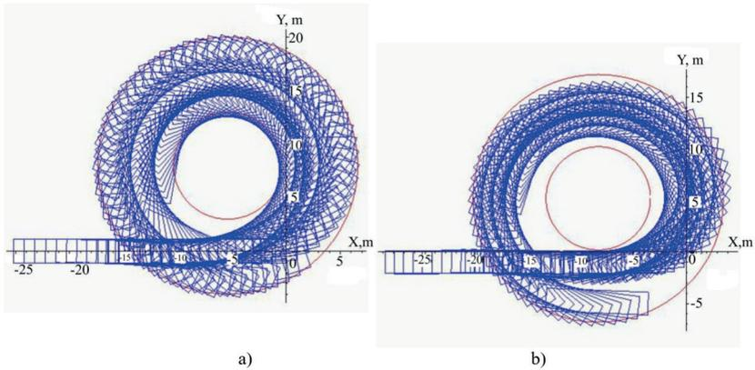
Fig. 8. Overall traffic lane of the metrobus with a speed 5 m/s:
