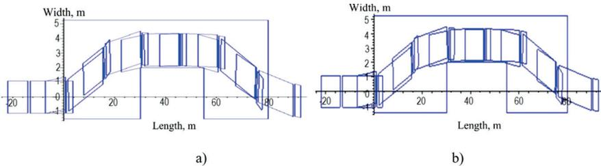
Fig. 9. Trajectories of the movement of the metrobus links with unruled second trailer a) and a driven second trailer b) when performing an ISO maneuver and speed 5 m/s
