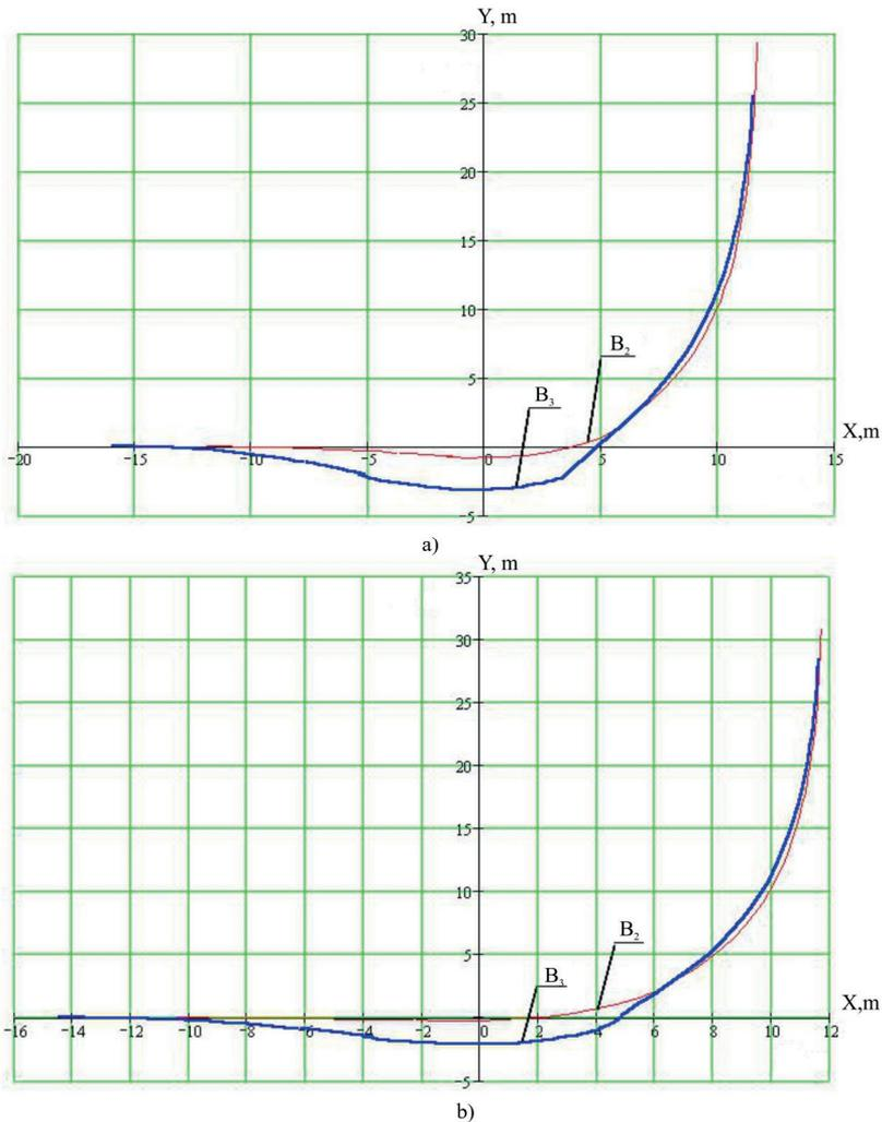
Fig. 6. Trajectories of the characteristic points of the first trailer  $B_2$  and a second trailer  $B_3$ :
