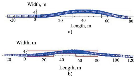
Fig. 10. Trajectories of the movement of the metrobus links with unruled second trailer a) and a driven second trailer b) when performing an ISO maneuver and speed 10 m/s
