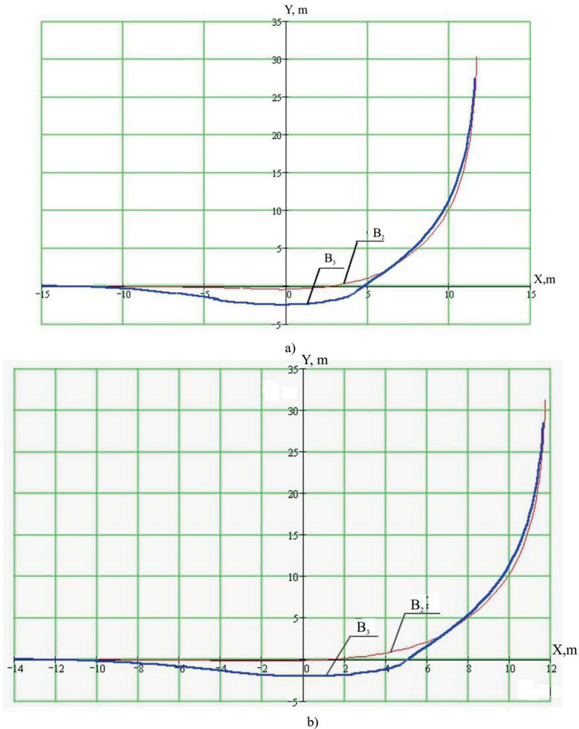
Fig. 5. Trajectories of the characteristic points of the first  $B_2$  trailer and the second managed trailer  $B_3$ :
