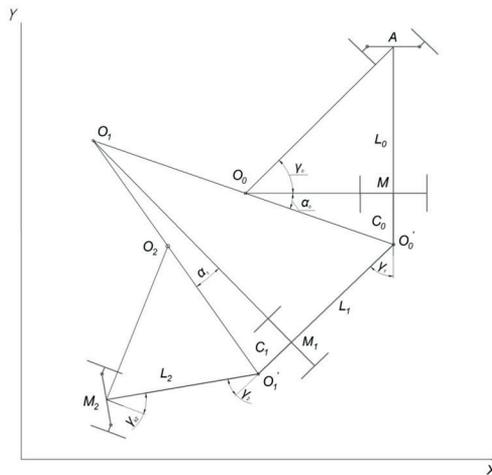
Fig. 2. The scheme of rotation of a three-lane metrobus with a controlled second trailer
