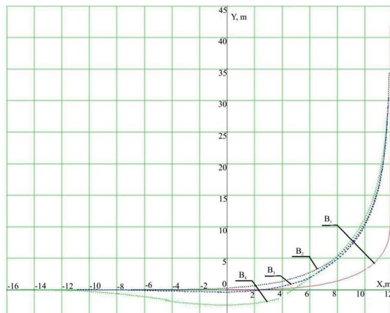
Fig. 4. Trajectories of the links points of the road train
