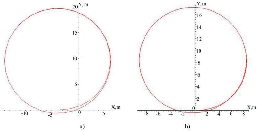
Fig. 7. The trajectories of the center of mass of the metrobus with a speed 5 m/s:
