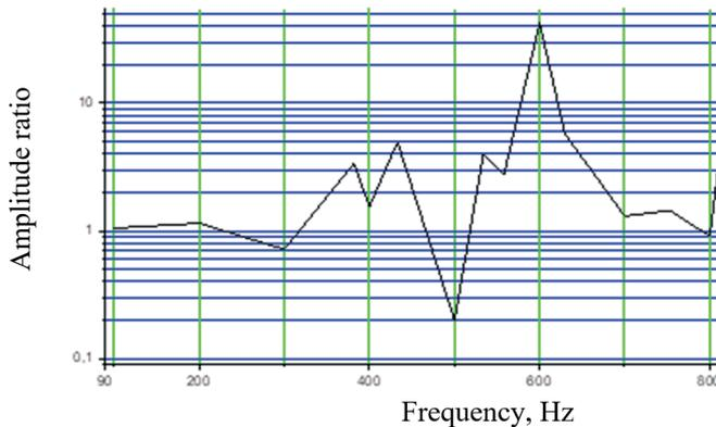
**Fig. 7. The ratio of the amplitudes of the acceleration of the transducer measuring head and the housing to the corresponding excitation frequencies**
