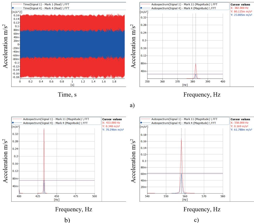
**Fig. 6.** Graphs of the three-way acceleration and spectral density of the housing and measuring head of a linear transducer with sinusoidal excitation (a - 382 Hz; b - 433 Hz; c - 558 Hz); in the Z direction (Figure 1):
