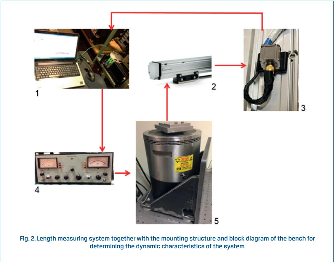
Fig. 2. Length measuring system together with the mounting structure and block diagram of the bench for determining the dynamic characteristics of the system
