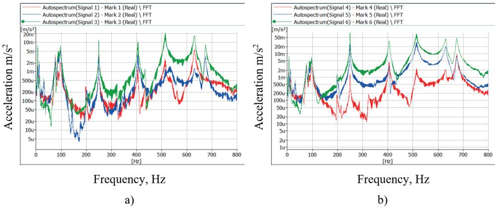
**Fig. 4.** Length measurement systems, when the structure is excited by shock excitation in the Y direction (Figure 1), graphs of the three-way acceleration spectral density of the housing and measuring head: a) housing (red - Y direction; blue - Z direction; green - X direction) oscillations; b) vibrations of the linear converter head (red - Y direction; blue - Z direction; green - X direction)
