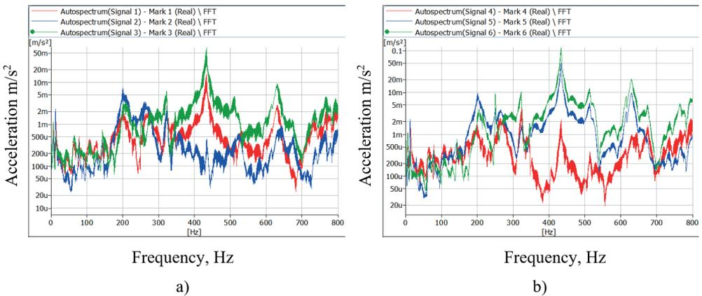
**Fig. 5.** Length measurement systems, when the structure is excited by shock excitation in the X direction (Figure 1), graphs of the three-way acceleration spectral density of the housing and measuring head: a) housing (red - Y direction; blue - Z direction; green - X direction) oscillations; b) linear converter heads (red - Y direction; blue - Z direction; green - X
