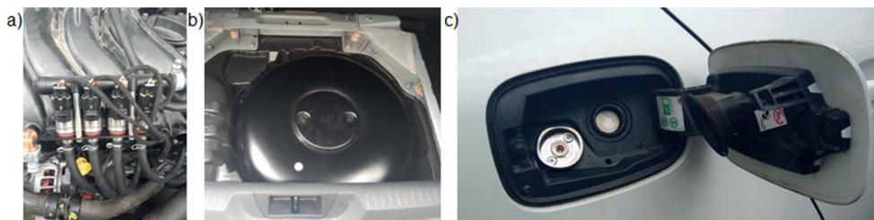
Fig. 2. The LPG system components, a) LPG injectors, b) LPG tank, c) LPG refuelling valve
