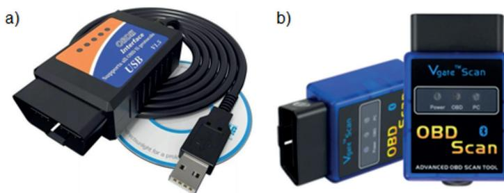
Fig. 6. a) OBD interface with USB plug, b) OBD interface communicating via Bluetooth
