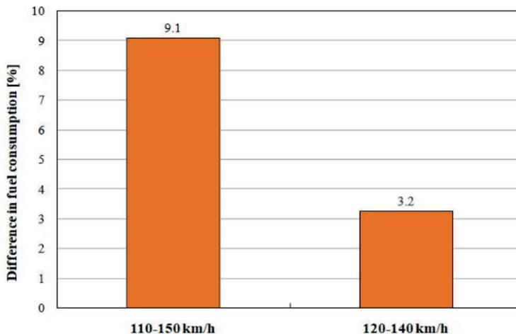
Fig. 9. Percentage change in vehicle fuel consumption in relation to the reference test drive at  $V = 130 \text{ km/h}$
