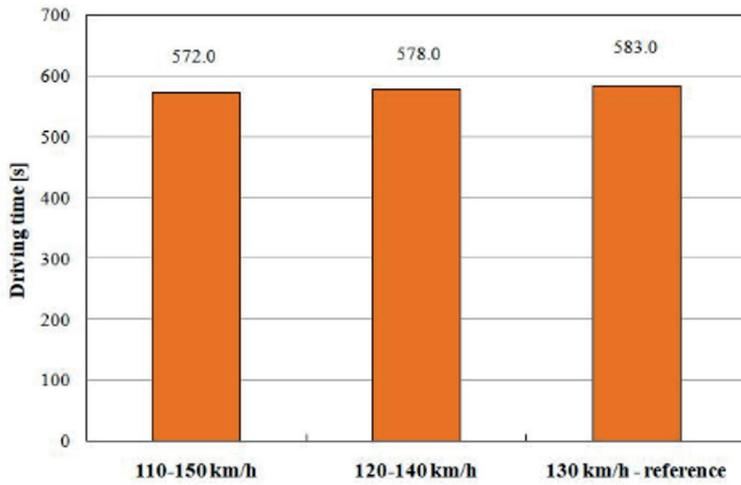
Fig. 4. Travel time through the test road section in relation to the different speed ranges used
