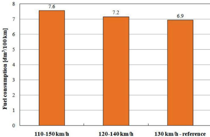
Fig. 8. The test vehicle fuel consumption values for each of the test drives
