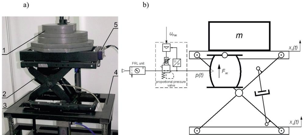
Fig. 7. General view (a) and diagram (b) of experimental stand: 1 – mass load, 2 – bellows cylinder, 3 – scissor-type working machine, 4 – vibrating table, 5 – laser displacement sensor
