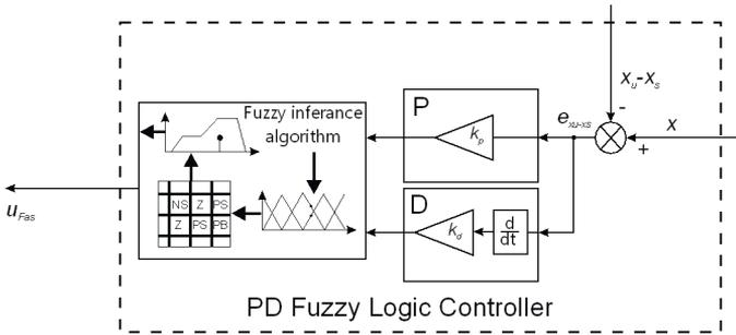
Fig. 5. Diagram of PD Fuzzy Logic Controller
