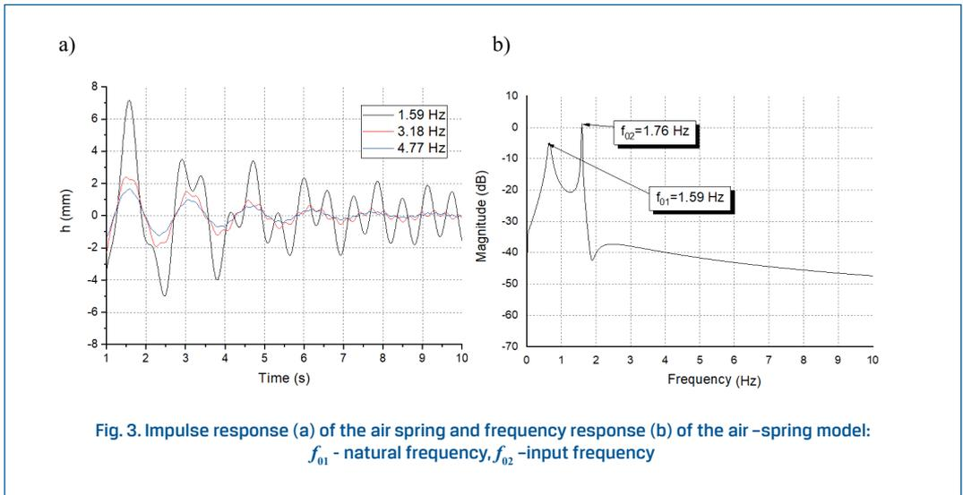
In the simulation system of the bellows actuator model, a decrease in amplitude is observed in the natural frequency range  $f_{01}$  as well as in the original input frequency range  $f_{02}$ . The natural frequency of the mechanical system was determined by the Fast Fourier Transform (FFT) (Figure 3b) from the impulse response (Figure 3a).
