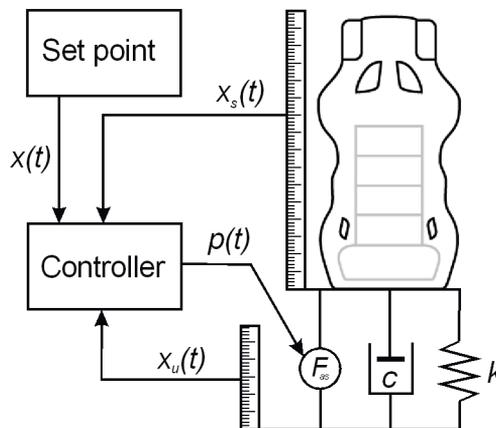
Fig. 4. Block diagram of the active seat suspension control system
