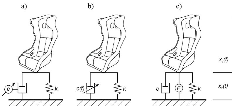
Fig. 1. Block diagram of the active seat suspension control system: a) adjustable, b) semi-active, c) active
