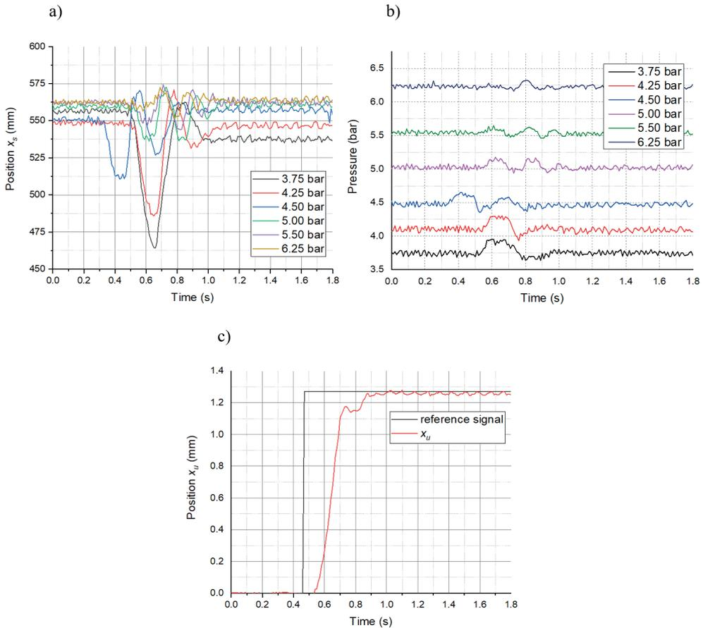
**Fig. 8. Dynamic characteristics of displacement of the vibro-insulated mass  $x_s(t)$  (a), pressures (b) and floor displacement  $x_u(t)$  (c)**
