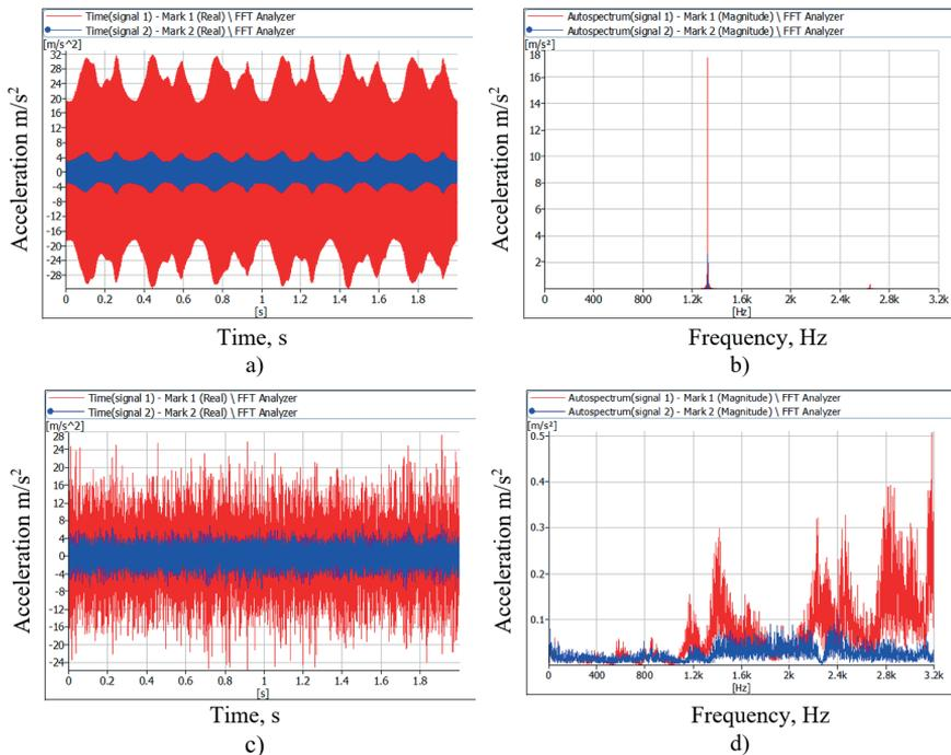
**Fig. 4** Temporary (Z-direction) acceleration curves of the acceleration of the high-resolution coded precision angle encoder system at 2 points (Figure 2: red curve of the vibrator base and blue curve of the encoder housing) a) for sinusoidal excitation 1322 Hz; c) for random excitation, i.e. white noise and corresponding frequency acceleration plots; b) for 1322 Hz sinusoidal excitation; d) for white noise)
