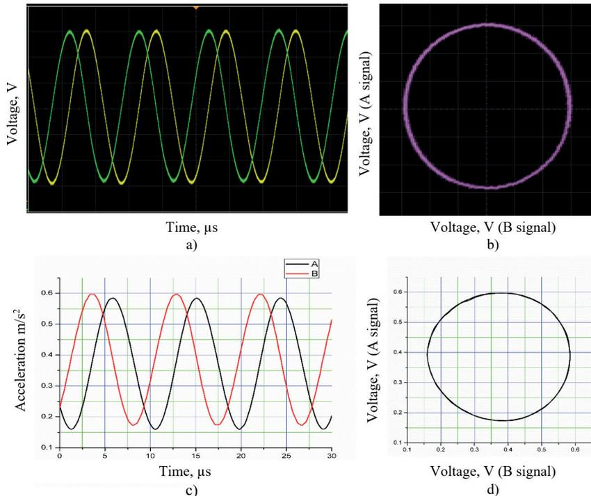
**Fig. 5** The output signals A (sine) and B (cosine) of the high-resolution coded precision angle encoder are presented as a function of time and in the form of a Lissajous curve: a) when the encoder shaft rotates at a constant speed and has no vibration effect; b) when the sensor is subjected to random excitation and white noise; c) presented in the acceleration curves at the same conditions as a); d) presented in the voltage signals influence at the same conditions as b)
