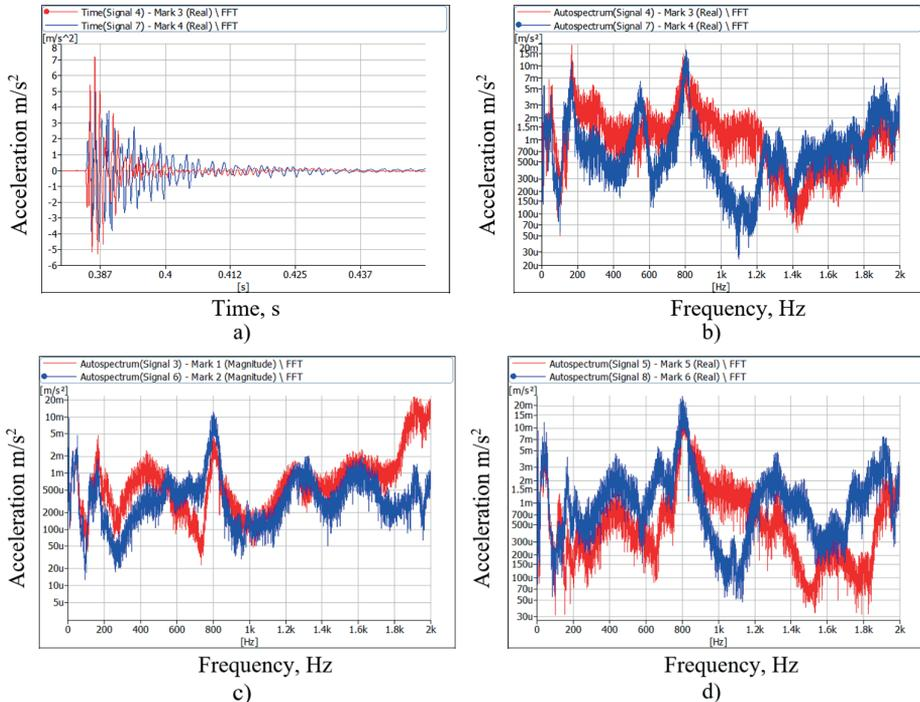
**Fig. 3** Time-domain a) (Y-direction) acceleration and frequency acceleration curves of the 2-point high-resolution coded precision angle encoder system (Figure 2b vibrator base red curve and encoder body blue curve): b) – Y direction, c) – Z direction and d) – X direction
