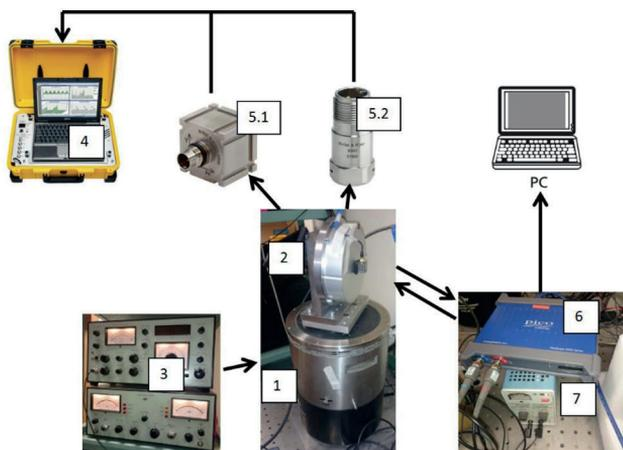
Fig. 2. High-resolution code precision angle encoder system with the mounting structure for determining the dynamic characteristics of the system
