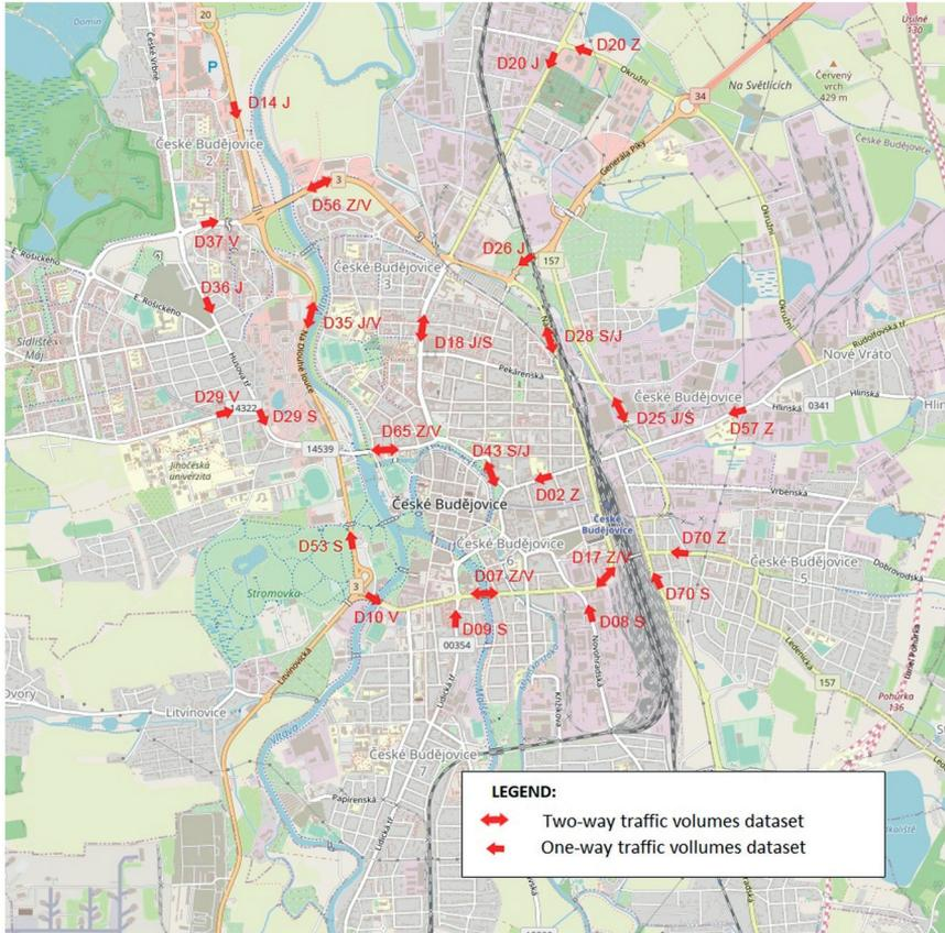
Fig. 1. Diagram of the road network in the city with the location of 28 traffic monitoring detectors
