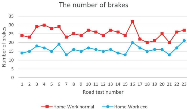
Fig. 2. The number of brake applications during road tests
