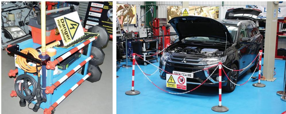
Fig. 3. Electric shock protection measures in the workshop [51]
