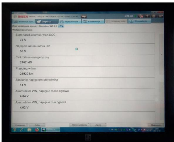
**Fig. 8. Bosch KTS software screen**
