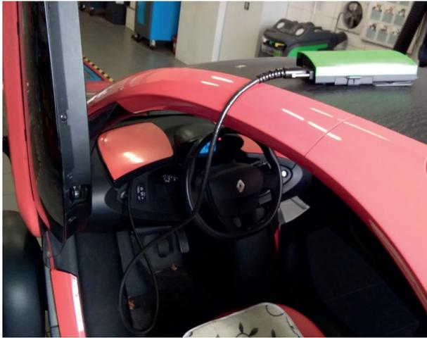
Fig 6. Bosch KTS connected to the vehicle
