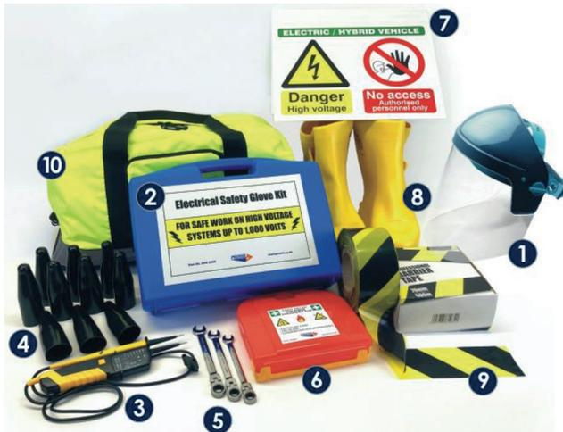
Fig. 1. An example of a set of equipment for a workshop servicing electric vehicles [50]
