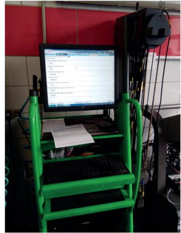
Fig. 7. Bosch KTS diagnostic device
