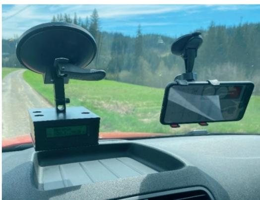
Fig. 2. The location of the measurement tool [XL Meter™ Pro – left; smartphone – right].
