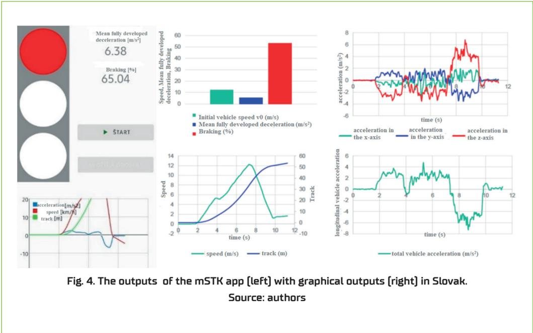
Immediately after the measurement, the mobile application calculates the results of the brake test, namely mean fully developed deceleration as defined by ECE Regulation No. 13, as well as the braking rate, which is defined by:
