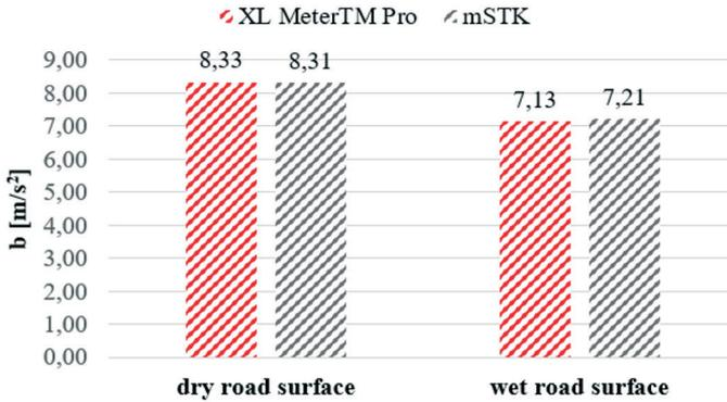
Fig. 6. Average full braking deceleration for wet and dry roads on both surfaces. Source: authors
