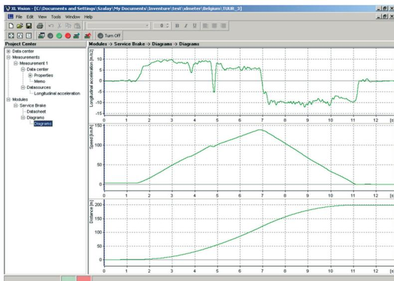
Fig. 3. The progress of the measurement in the graphical display in the program XL Vision™.
