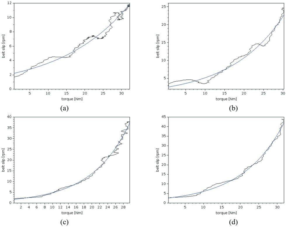
**Fig. 8. Measured belt slip  $\omega_s$  [—] and calculated approximation lines  $\omega'_s$  [—] as a function of resistance torque: [a]  $F_0=500$  N, [b]  $F_0=250$  N, [c]  $F_0=125$  N, [d]  $F_0=75$  N**
