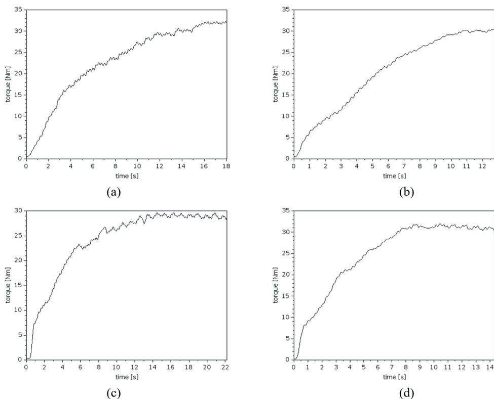
**Fig. 4. Measured courses of resistance torque  $M_{res}$  in transmission:**
