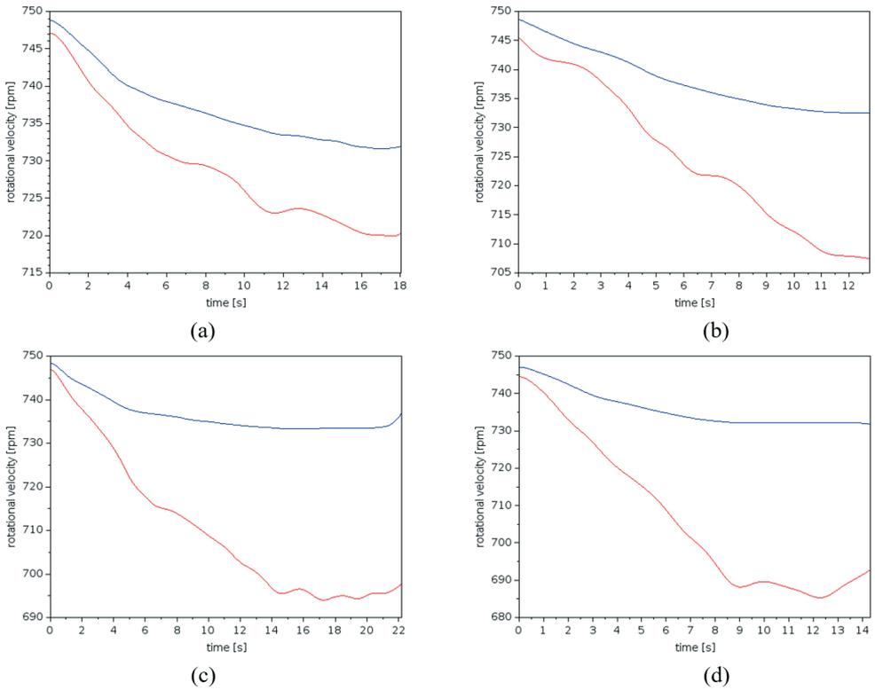
**Fig. 3. Measured courses of rotational velocities of pulleys  $\omega_1$  [—] and  $\omega_2$  [—]:**
