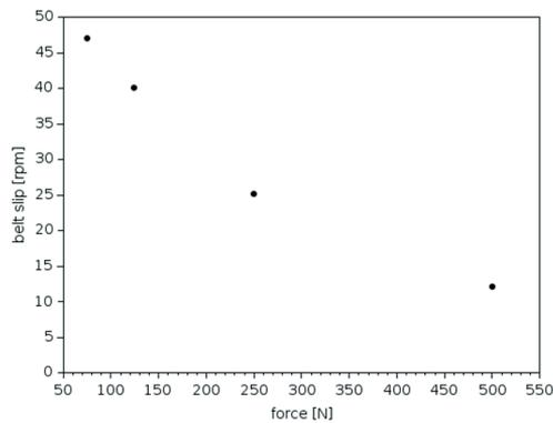
Fig. 7. Values of maximum measured values of belt slip  $\omega_s$  in assumed cases of preload force  $F_0$
