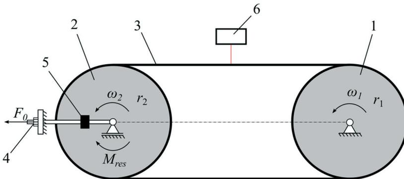
Fig. 2. Scheme of the measured system with a belt transmission
