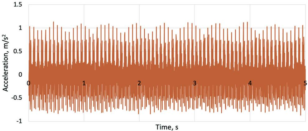
**Fig. 10. Time histories of the accelerations recorded on the motorcycle handlebars during the test performed at an excitation frequency of 14 Hz**
