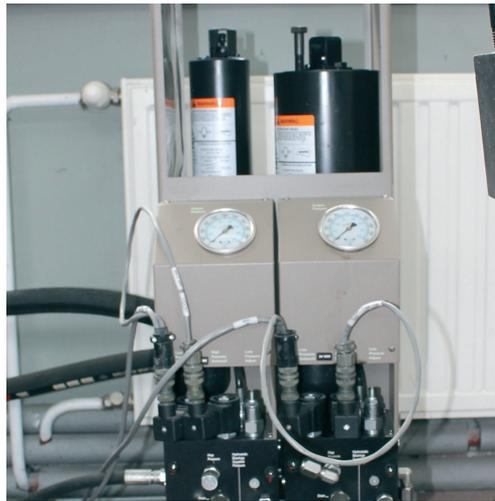
Fig. 2. Hydraulic distributor
