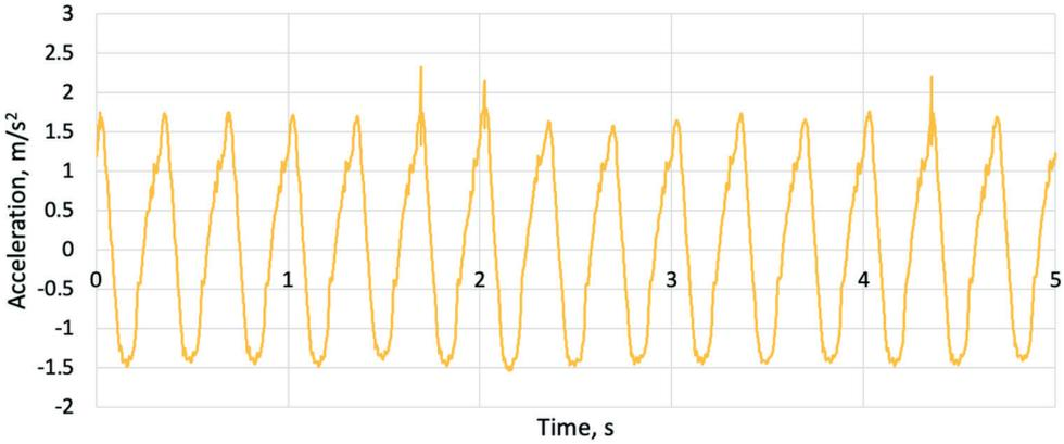
**Fig. 9. Time histories of the accelerations recorded on the motorcycle seat during the test carried out at an exciting frequency of 3 Hz**
