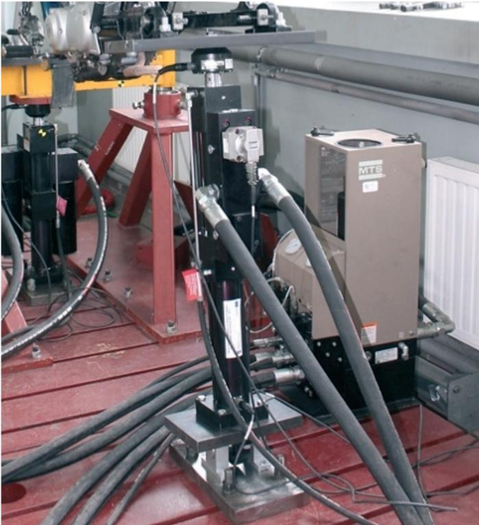
**Fig. 7. Electro-hydraulic pulsator with joint and plate enabling the installation of motorcycle control arms**
