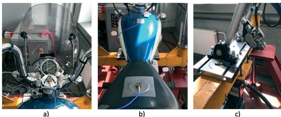
**Fig. 8. Location of individual acceleration sensors;
