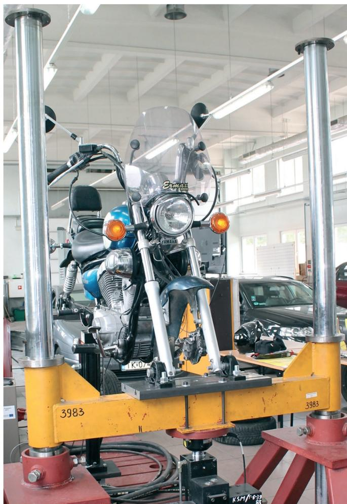
**Fig. 6. Guide system with motorcycle front fork mounting unit**
