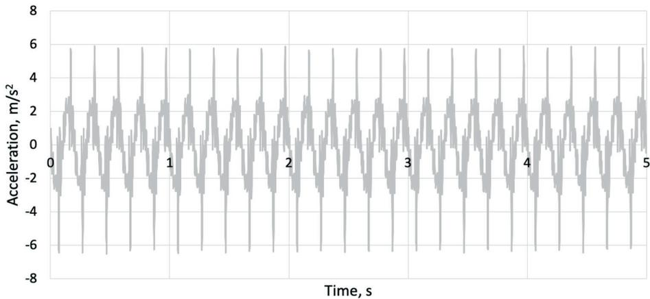
**Fig. 11. Time histories of the accelerations recorded on the front suspension mounting plate during the test carried out at an excitation frequency of 5 Hz**
