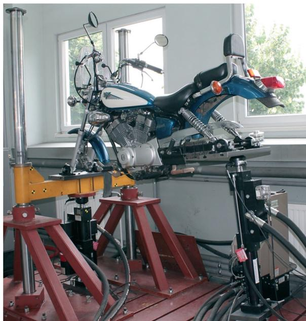
**Fig. 1. Motorcycle vibration test stand**
