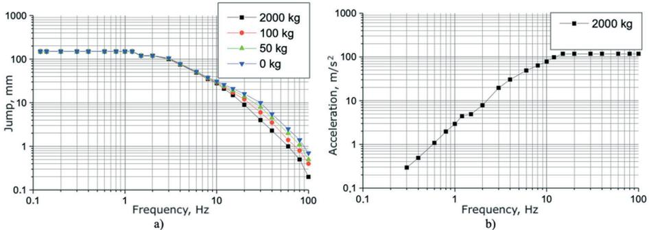
Fig. 3. External characteristics of pulsators: a) jump – frequency, b) acceleration – frequency
