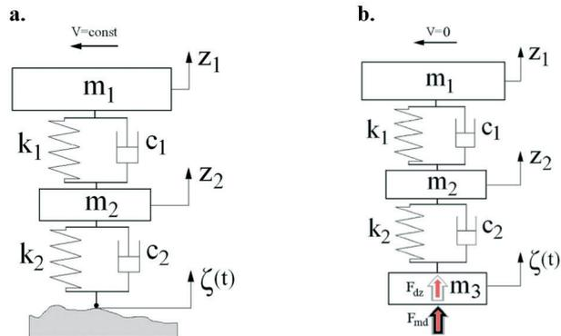
**Fig. 3. Linear 'quarter-car' model, where [a] is general version, [b] is version dedicated to the vehicle on a diagnostic tester ( $V=0$ ; the vibration plate inertia is considered)**
