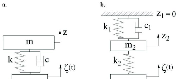
**Fig. 4. Simplified 'quarter-car' models, where [a] is 1DOF system obtained by disregarding the 'unsprung mass' and adopting an equivalent suspension elasticity [elasticity of the suspension and tire arranged in series], [b] is another 1DOF system intended for the situation where the 'sprung mass' is immobile**
