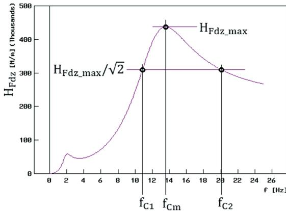
**Fig. 5. The 'peak-picking' method, variants 'Calvo 1' and 'Calvo 2'. The absolute value of transmittance  $H_{Fdz}$  of force  $F_{dz}$  in the area around its maximum  $H_{Fdz\_max}$  is analysed.  $f$  represents the Hertz frequency**
