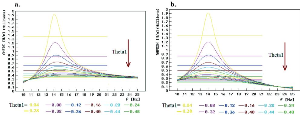
**Fig. 7.** Illustration of the applicability of the ‘Calvo 1’ and ‘Calvo 2’ methods to the analysis carried out close to the 2<sup>nd</sup> resonance frequency. Analysed are the absolute values of transmittances  $H_{FdZ}$  [a] and  $H_{Fmd}$  [(b) - related to the tire-exciter contact force and to its measured value, respectively, and denoted by AHFDZ and AHFDZM in the graphs] close to their maximums.
