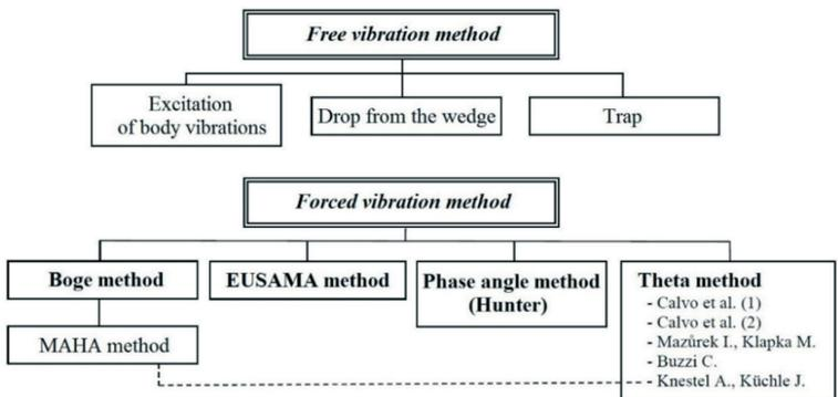
Fig. 1. On-vehicle methods of examining shock absorbers' condition
