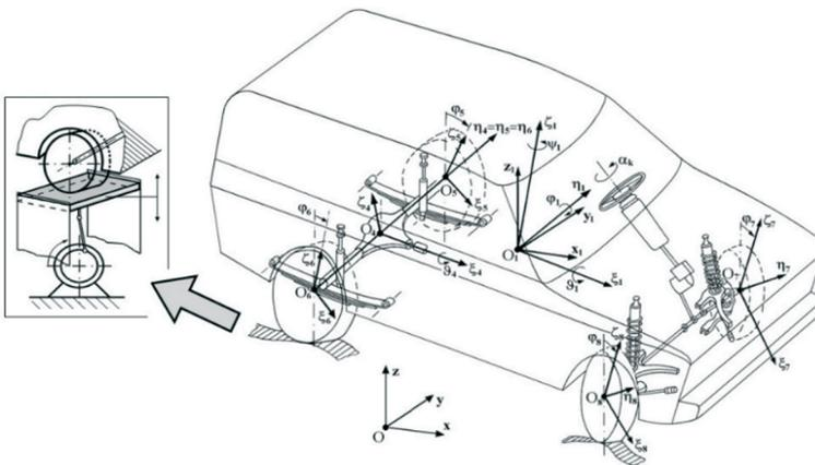
**Fig. 2. 3D model of vehicle dynamics with 14 DOF. Kinematic excitation in a form typical for the EUSAMA method applied to freely chosen vehicle wheel [16]**
