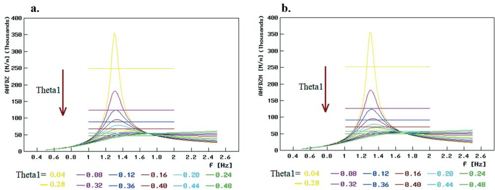
**Fig. 6. Illustration of the applicability of the ‘Calvo 1’ and ‘Calvo 2’ methods to the analysis carried out close to the 1<sup>st</sup> resonance frequency. Analysed are the absolute values of transmittances  $H_{Fdz}$  [a] and  $H_{Fmd}$  [(b) - related to the tire-exciter contact force and to its measured value, respectively, and denoted by AHFDZ and AHFDZM in the graphs] close to their maximums.**
