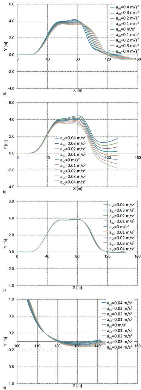
**Fig. 2. Trajectories of movement of the car; a) variant 1, b) variant 2, c) variant 3, d) a fragment of variant 3 enlarged in the interest area**
