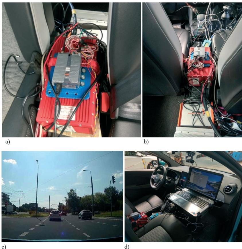
**Fig. 1. Picture from the test object, a) and b) view of the OXTS RT 3002 apparatus installed in the car, c) view from the vehicle during test, d) view from inside of the vehicle**
