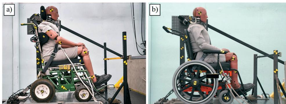
**Fig. 4. Example of tiedown/securement system testing: [a] surrogate wheelchair [15], [b] wheelchair frontal-impact testing [8]**
