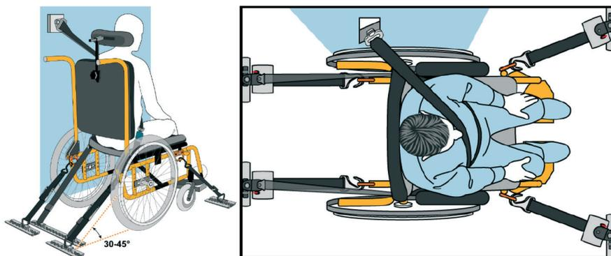
Fig. 1. Wheelchair Tie-down and Occupant Restraint System [18]
