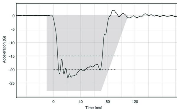
**Fig. 5. Typical 30-mph sled deceleration pulse [20]**
