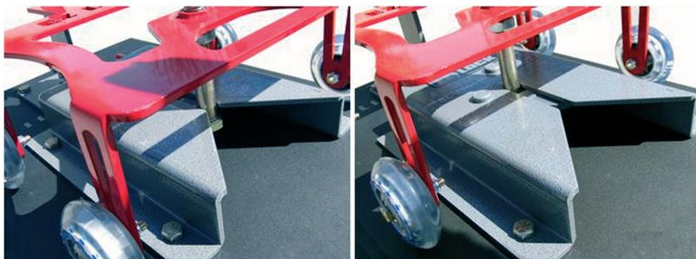
**Fig. 2. The EZ Lock Wheelchair Docking System [7]**
