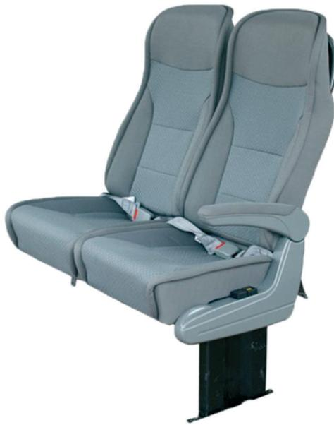
**Fig. 2. Seats with two-point seat belts**
