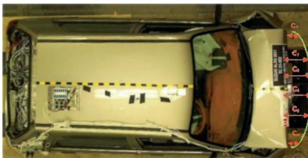
**Fig. 6. Frontal deformation with method of measurements**
