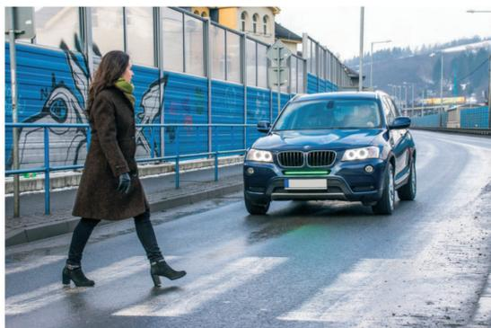
**Fig. 4. Vehicle braking information by illuminating the front brake light before a pedestrian crossing**
