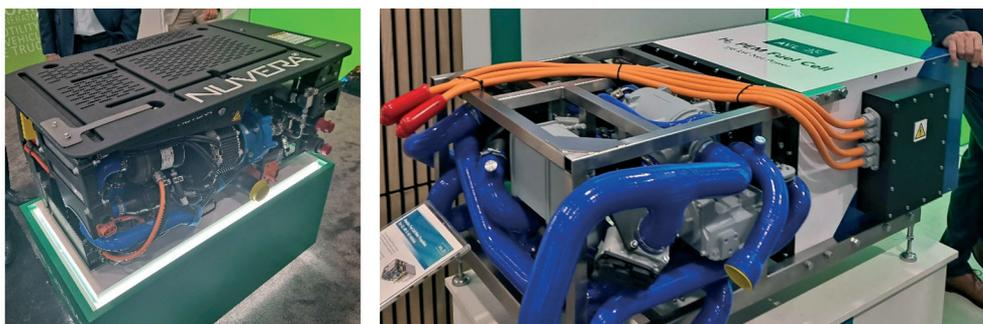
Fig. 13. Fuel cell system: [a] by Nuvera; [b] by AVL
