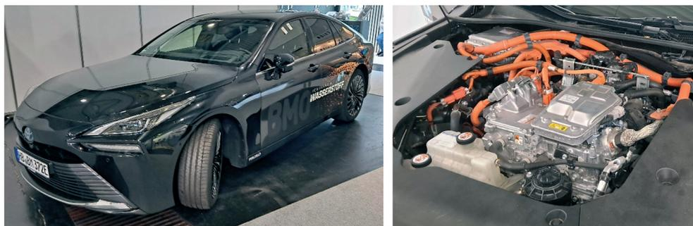
Fig. 12. Toyota Mirai powered by hydrogen: [a] view of the vehicle; [b] drive system
