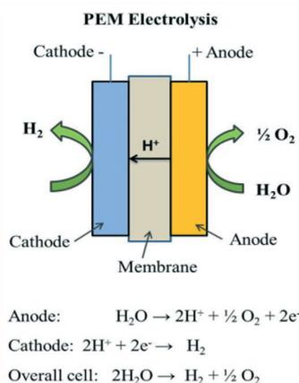
**Fig. 1. Construction of a single electrolyser cell with a PEM membrane [47]**
