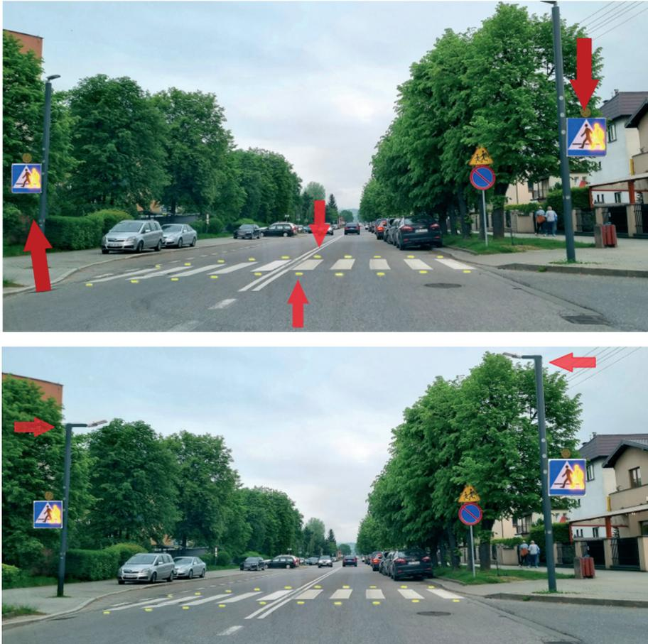
**Fig. 16. The visualisation of the pedestrian crossing at Lwowska Street with the use of mechatronic systems**
