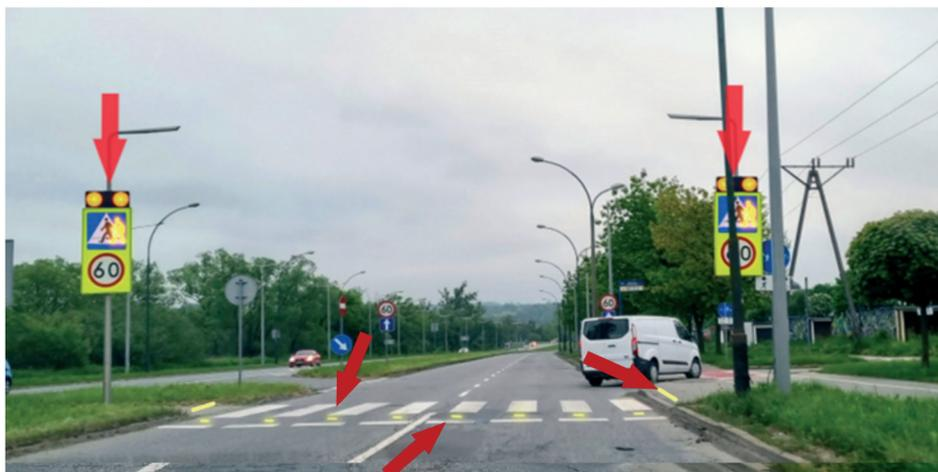
**Fig. 17. The visualisation of the pedestrian crossing at Aleje Piłsudskiego with the use of mechatronic systems**
