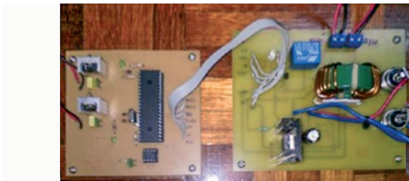
Fig. 10. Boost converter with control circuit
